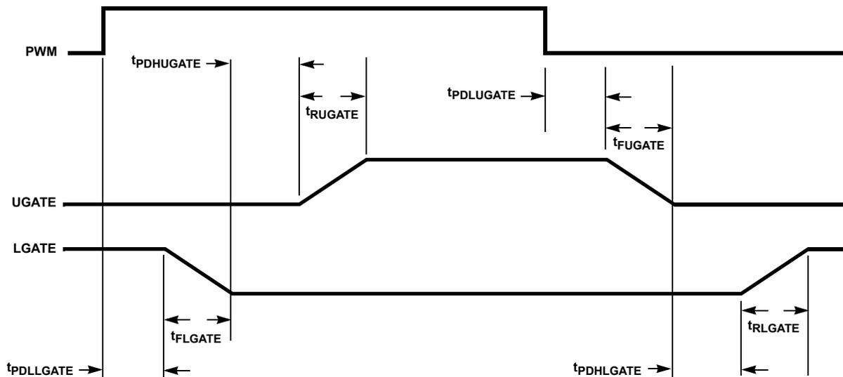
A falling transition on PWM indicates the turn-off of the upper MOSFET and the turn-on of the lower MOSFET. A short propagation delay [ $t_{PDLUGATE}$ ] is encountered before the upper gate begins to fall [ $t_{FUGATE}$ ]. Again, the adaptive shoot-through circuitry determines the lower gate delay time,  $t_{PDHLGATE}$ . The PHASE voltage is monitored and the lower gate is allowed to rise after PHASE drops below 0.5V. The lower gate then rises [ $t_{RLGATE}$ ], turning on the lower MOSFET.
