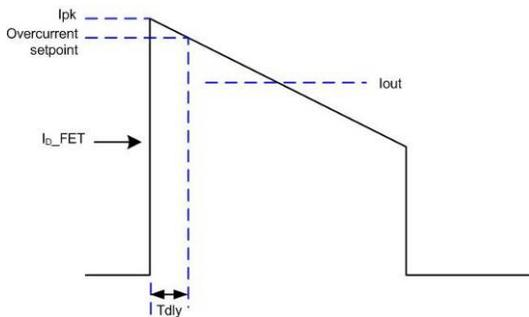
**Figure 9. Overcurrent waveform**
