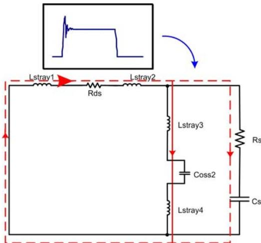
Figure 11. Snubber Circuit
