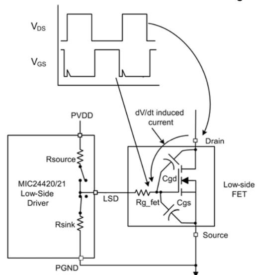
Figure 6. dV/dt induced turn-on of the low-side MOSFET
