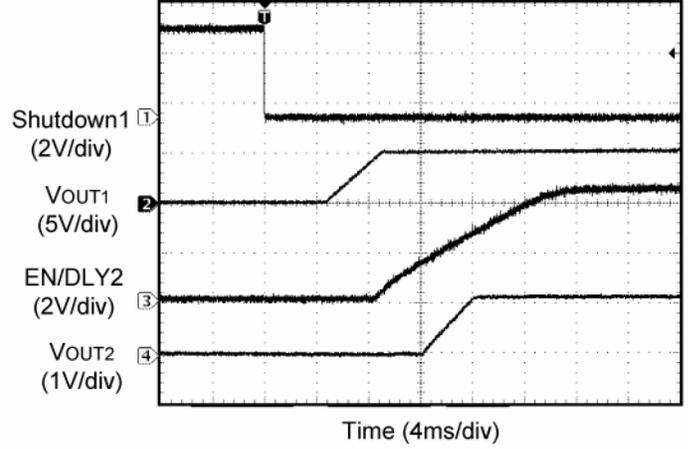
**Startup Into Overload (1Ω on 5V output)**
