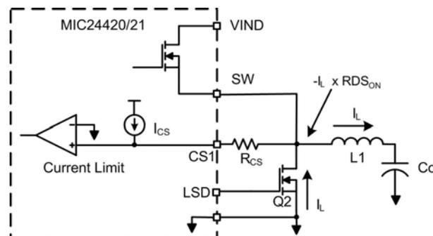
Figure 7. Over-current Circuit
