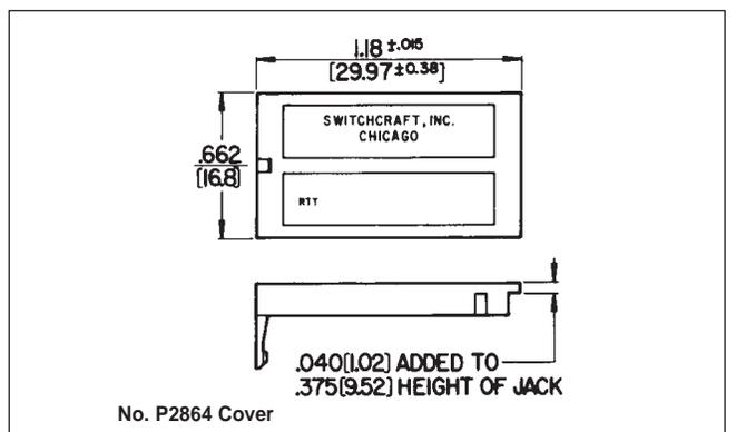
DIMENSIONS ARE FOR REFERENCE ONLY  $\frac{\text{Inch}}{\text{(mm)}}$
