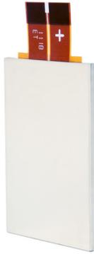
At 2 and 3 mm thin, type ULP offers the highest energy density available in a low profile aluminum electrolytic. It's ideal for the lowest profile circuits where high capacitance is needed for bulk storage. Look to type ULP to replace arrays of SMT solid tantalum capacitors.
