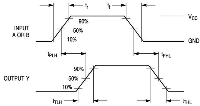
Figure 1. Switching Waveforms
