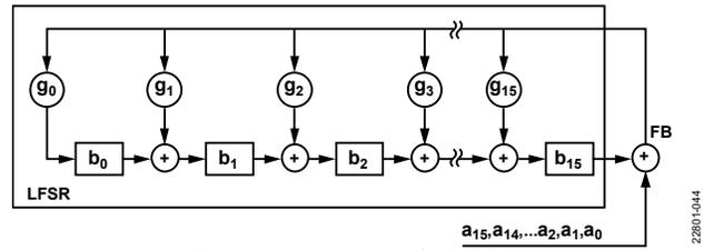
Figure 43. LFSR Generator Used for CRC Calculation
