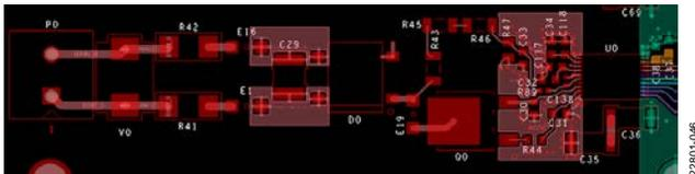
Figure 45. ADE1201 Circuit Board, Top Layer
