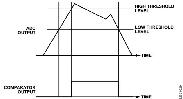
Figure 25. Comparator Behavior in Hysteretic Output Mode
