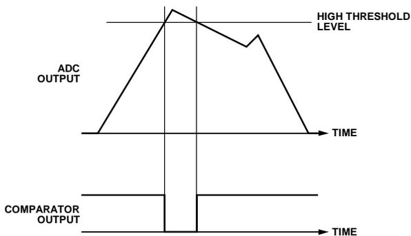
Figure 28. Comparator Behavior in LT Output Mode
