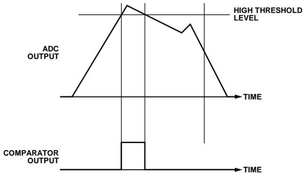
Figure 27. Comparator Behavior in GT Output Mode
