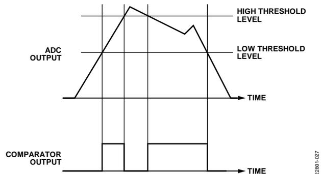
Figure 26. Comparator Behavior in Midrange Output Mode
