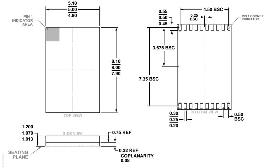
Figure 50. 20-Lead Land Grid Array [LGA] (CC-20-5)
