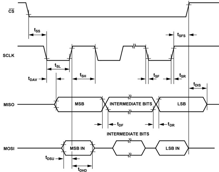
Figure 3. SPI Timing
