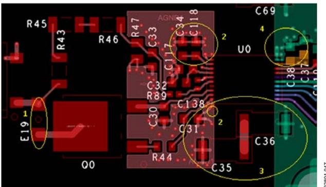
Figure 46. Close Up of the ADE1201 Support Circuitry
