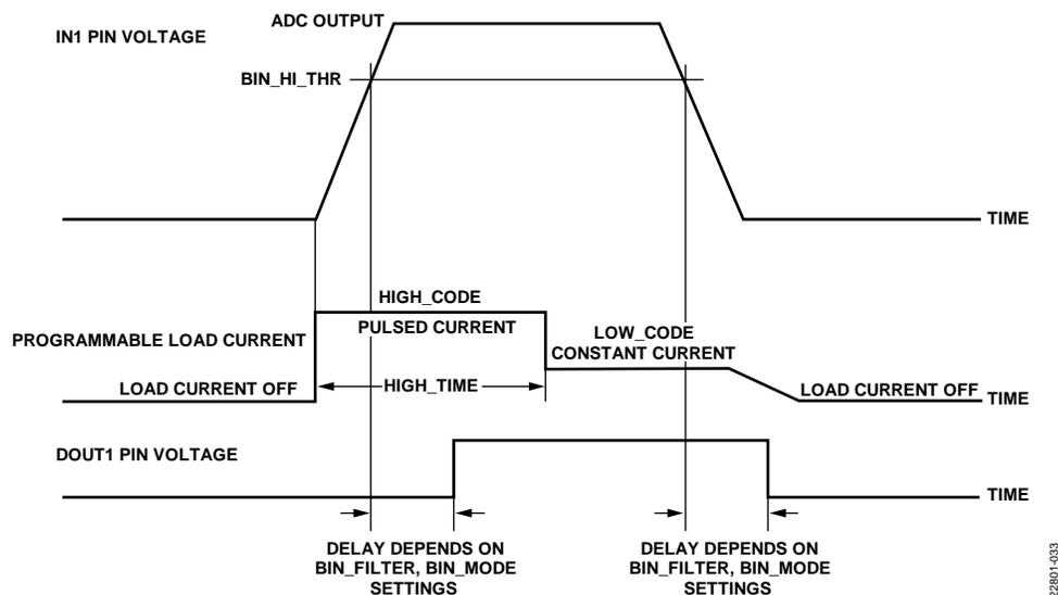
Figure 32. Programmable Load Current Waveform in High Idle Mode
