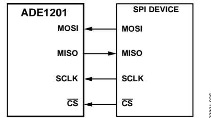
Figure 35. Connecting the SPI to an SPI Device
