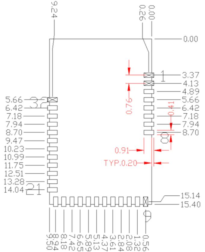
Table 3 provides the center location for each solder pad on the CYBLE-224110-00. All dimensions are referenced to the center of the solder pad. Refer to Figure 6 for the location of each module solder pad.
