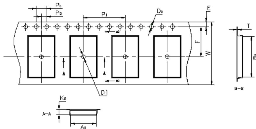
Figure 11 details the orientation of the CYBLE-224110-00 in the tape as well as the direction for unreeling.
