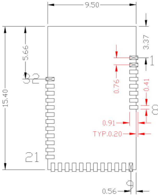
Figure 5. Module Pad Location from Origin
