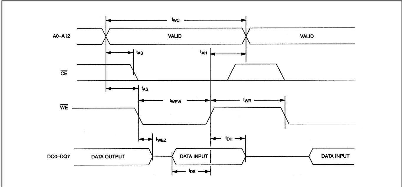
**WRITE CYCLE TIMING— $\overline{CE}/\overline{CE2}$ -CONTROLLED (See Note 5)**
