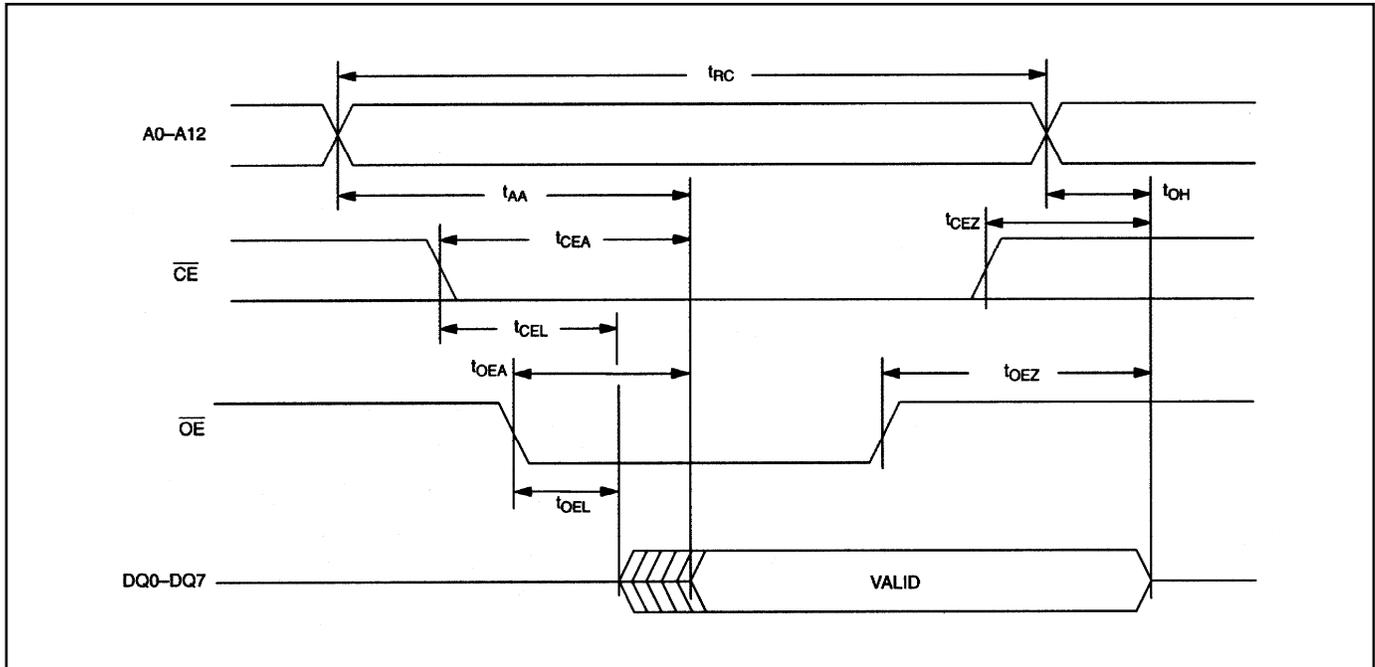
**AC CHARACTERISTICS—WRITE CYCLE (5V)**(V<sub>CC</sub> = 5.0V ±10%, T<sub>A</sub> = Over the Operating Range.)
