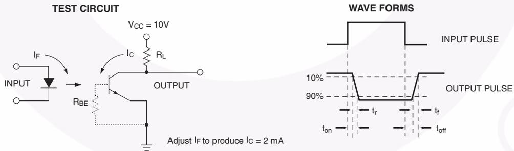
Figure 11. Switching Time Test Circuit and Waveforms
