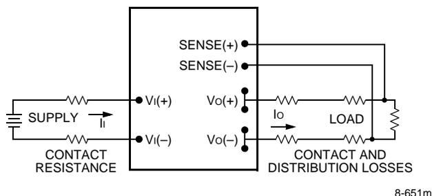
**Figure 12. Effective Circuit Configuration for Single-Module Remote-Sense Operation**
