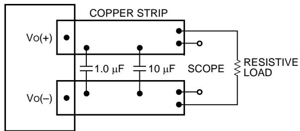
Note: Use a 1.0 µF ceramic capacitor and a 10 µF aluminum or tantalum capacitor. Scope measurement should be made using a BNC socket. Position the load between 51 mm and 76 mm (2 in. and 3 in.) from the module.
