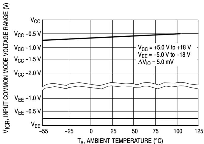
Figure 6. Input Common Mode Voltage Range versus Temperature
