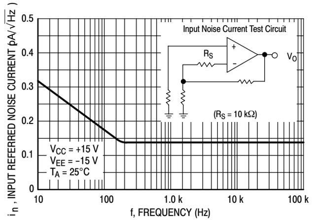
Figure 29. Input Referred Noise Current versus Frequency
