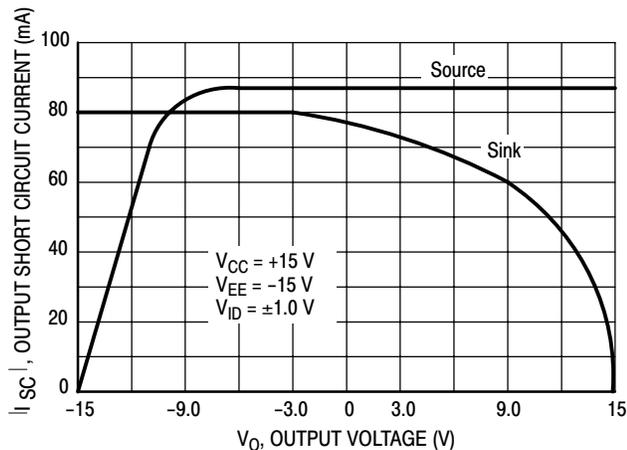
Figure 14. Output Short Circuit Current versus Output Voltage
