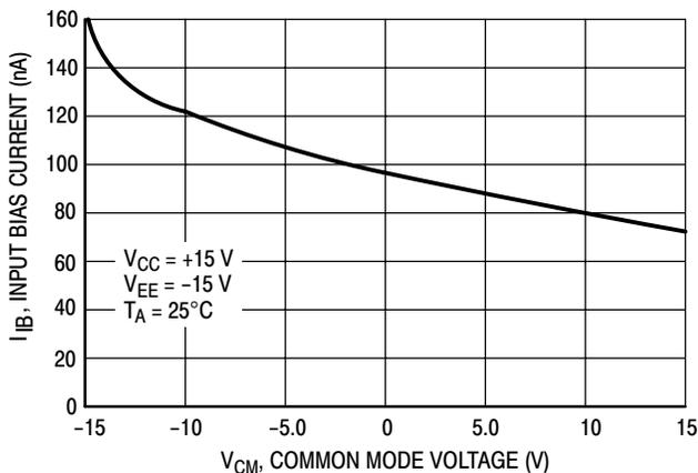
Figure 4. Input Bias Current versus Common Mode Voltage
