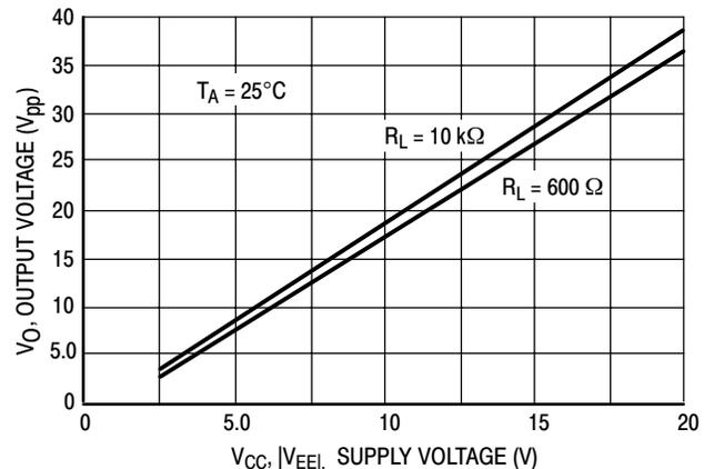
Figure 9. Output Voltage Swing versus Supply Voltage
