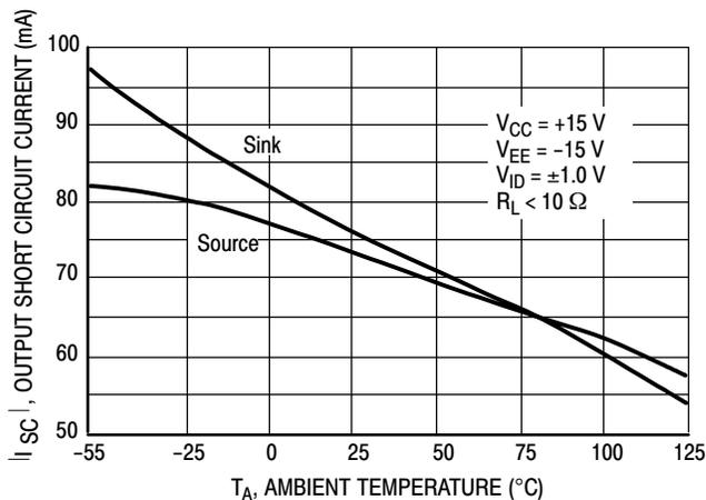
Figure 15. Output Short Circuit Current versus Temperature
