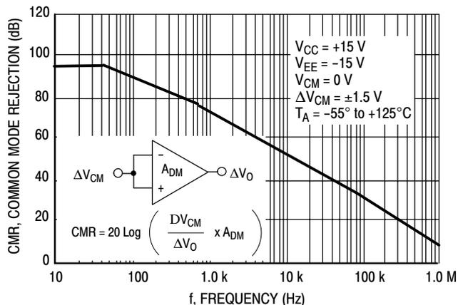
Figure 12. Common Mode Rejection versus Frequency Over Temperature
