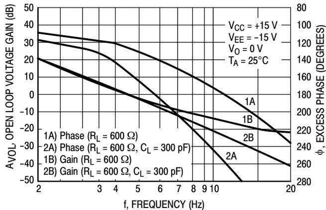
Figure 8. Voltage Gain and Phase versus Frequency
