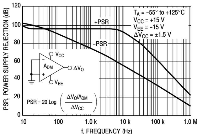
Figure 13. Power Supply Rejection versus Frequency Over Temperature
