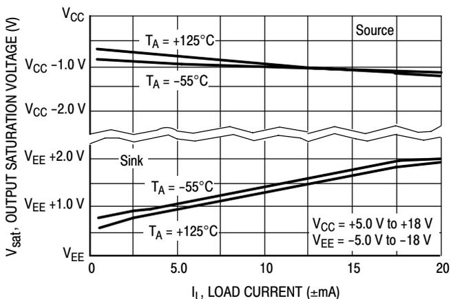
Figure 10. Output Saturation Voltage versus Load Current
