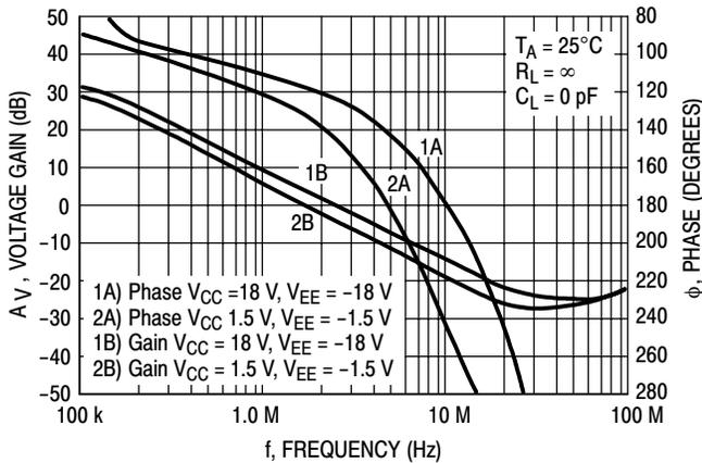
**Figure 20. Voltage Gain and Phase versus Frequency**
