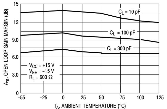
**Figure 21. Open Loop Gain Margin versus Temperature**
