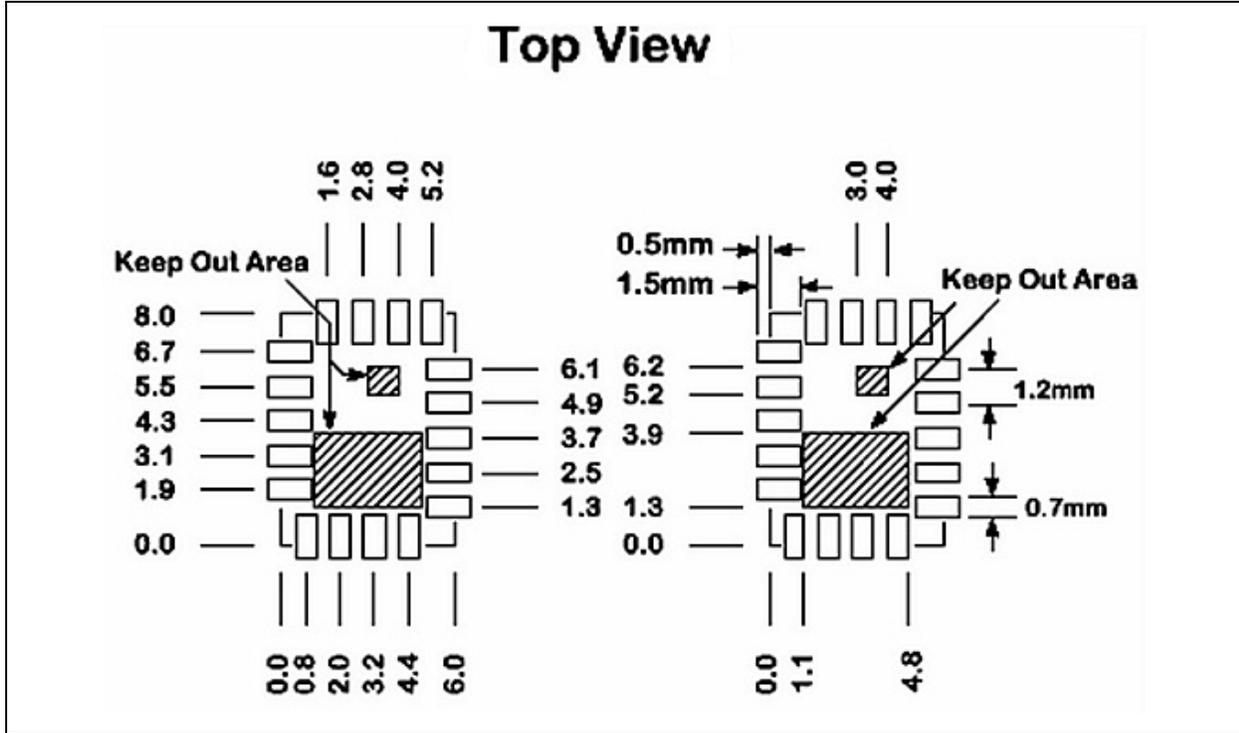
FIGURE 4-12: RN4871U RECOMMENDED PCB MOUNTING
