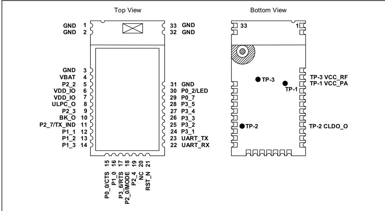
FIGURE 1-3: PIN DIAGRAM – RN4871U
