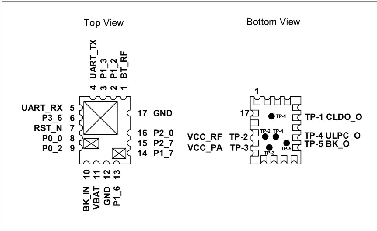
FIGURE 1-4: PIN DIAGRAM – RN4871
