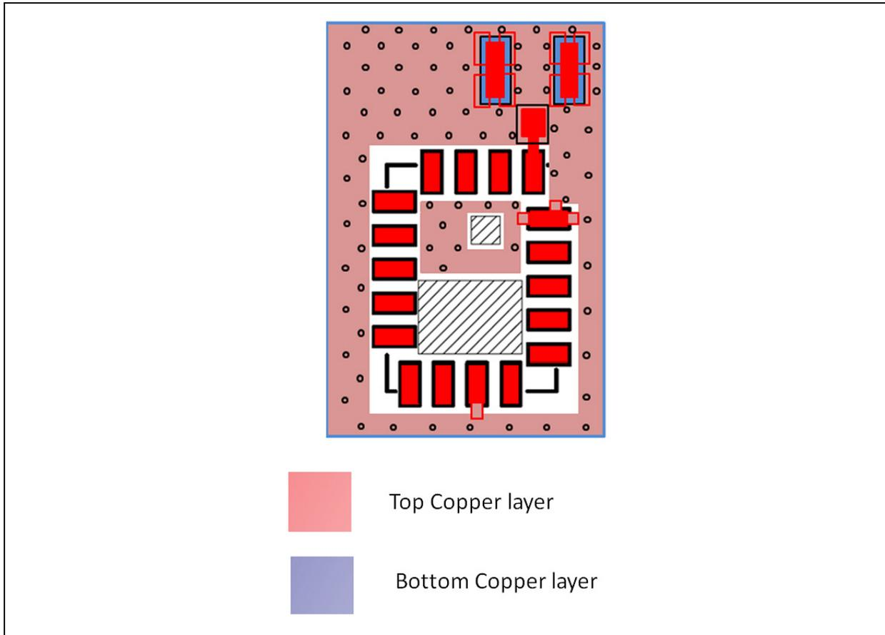
**FIGURE 4-13: RECOMMENDATIONS FOR PLACEMENT OF THE MODULE ON HOST PCB BOARD**
