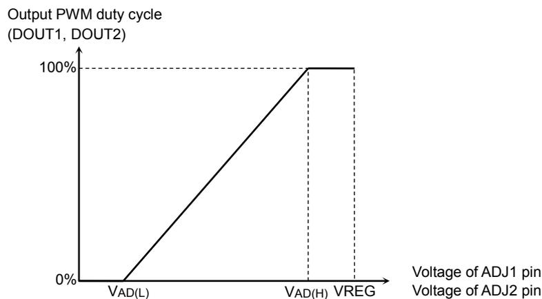
Note: Voltage setting of ADJ1 pin and ADJ2 pin should be set as follows; voltage of ADJ1 pin  $\leq$  voltage of ADJ2 pin. If it is set as follows; voltage of ADJ1 pin  $>$  voltage of ADJ2 pin, this function may not operate correctly.
