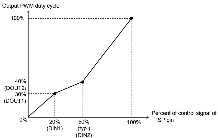
To set the above relation between the percent of control signal of TSP pin and the output PWM duty cycle, set the level of SEL\_ADJ pin and the voltage of ADJ0 pin, ADJ1 pin and ADJ2 pin shown below.
