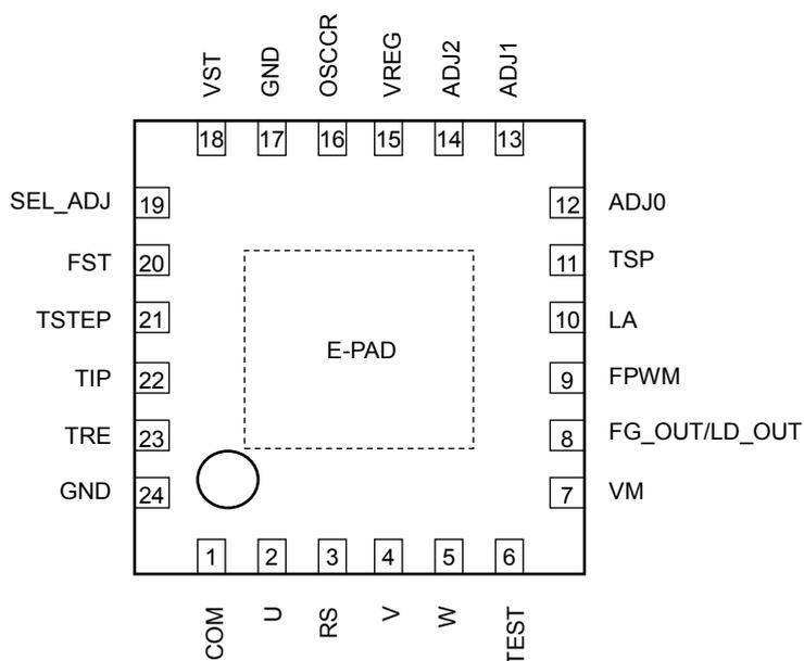
Note: Design the pattern in consideration of the heat design because the back side (E-PAD (2.6 mm×2.6 mm)) has the role of heat radiation. (A metal on the back side of a package (E-PAD) should be connected to GND because it is connected to the back of the chip in the package electrically.)
