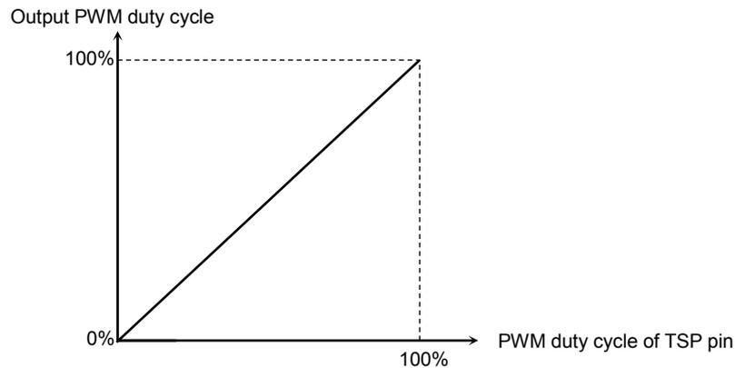
Note: The relation when ADJ1 pin and ADJ2 pin are connect to ground is shown above. For details of ADJ1 pin and ADJ2 pin, refer to 5.3
