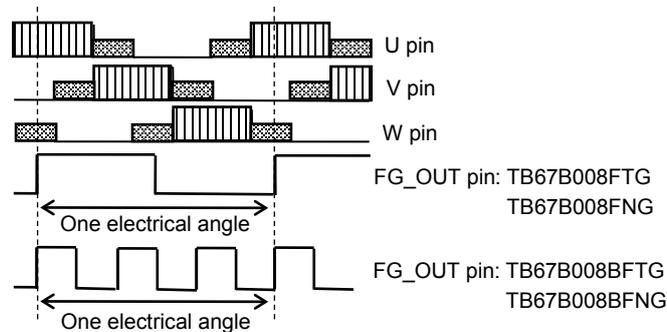
2)Rotation speed detection signal output pin: FG\_OUT pin
