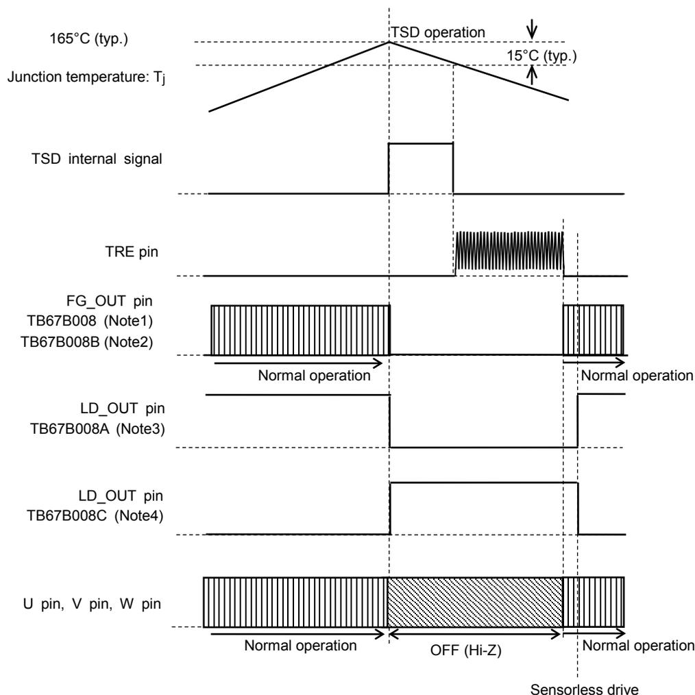
Note: The TSD circuit is activated if the absolute maximum junction temperature rating ( $T_j$ ) of 150°C is violated. Note that the circuit is provided as an auxiliary only and does not necessarily provide the IC with a perfect protection from any kind of damages.
