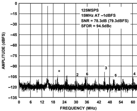
Figure 25. Single-Tone 16k FFT with  $f_{IN} = 15\text{ MHz}$ ,  $f_{SAMPLE} = 125\text{ MSPS}$ ,  $V_{REF} = 1.3\text{ V}$
