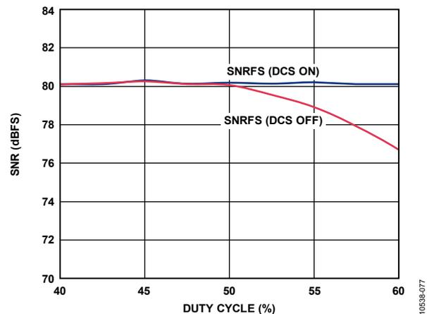
Figure 68. SNR vs. DCS On/Off,  $V_{REF} = 1.3V$
