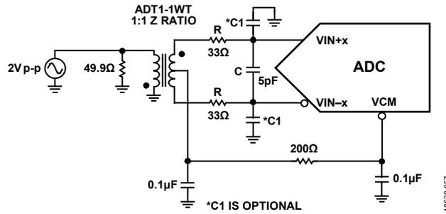
Figure 57. Differential Transformer-Coupled Configuration for Baseband Applications
