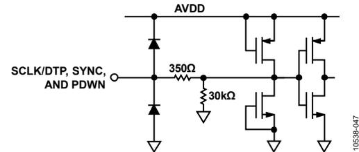
Figure 47. Equivalent SCLK/DTP, SYNC, and PDWN Input Circuit
