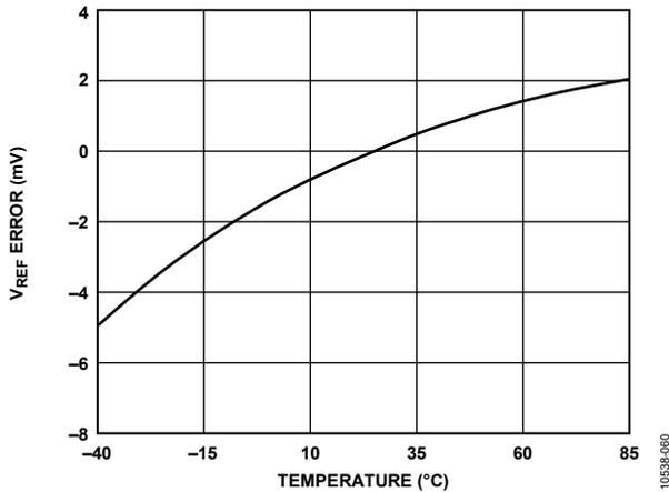
Figure 60. Typical  $V_{REF} = 1.0$  V Drift
