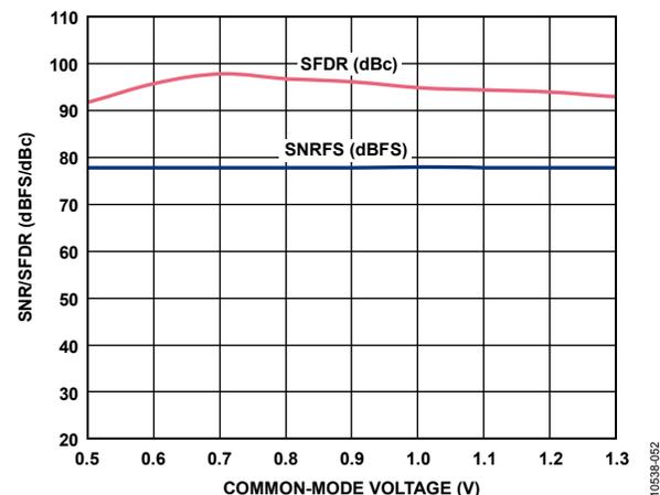
Figure 52. SNR/SFDR vs. Common-Mode Voltage,
