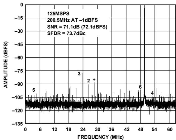
Figure 29. Single-Tone 16k FFT with  $f_{IN} = 200.5\text{ MHz}$ ,  $f_{SAMPLE} = 125\text{ MSPS}$ ,  $V_{REF} = 1.3\text{ V}$
