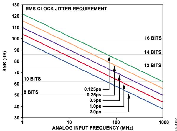
Figure 69. Ideal SNR vs. Input Frequency and Jitter
