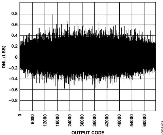
Figure 38. DNL,  $f_{IN} = 9.7$  MHz,  $f_{SAMPLE} = 125$  MSPS,  $V_{REF} = 1.3$  V
