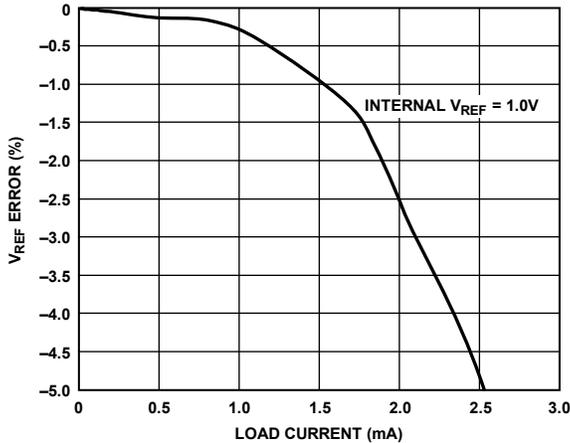
Figure 58.  $V_{REF} = 1.0\text{ V}$  Error vs. Load Current
