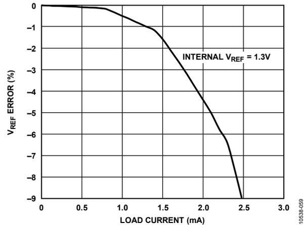
Figure 59.  $V_{REF} = 1.3\text{ V}$  Error vs. Load Current
