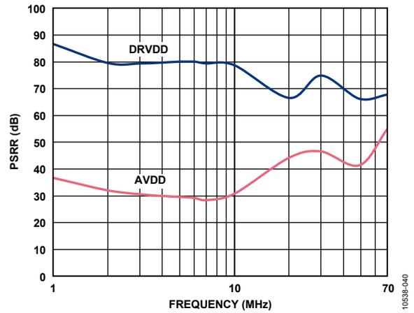
Figure 40. PSRR vs. Frequency,  $f_{SAMPLE} = 125$  MSPS,  $V_{REF} = 1.3$  V
