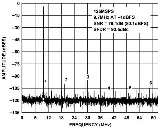
Figure 24. Single-Tone 16k FFT with  $f_{IN} = 9.7\text{ MHz}$ ,  $f_{SAMPLE} = 125\text{ MSPS}$ ,  $V_{REF} = 1.3\text{ V}$
