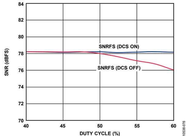
Figure 67. SNR vs. DCS On/Off,  $V_{REF} = 1.0V$
