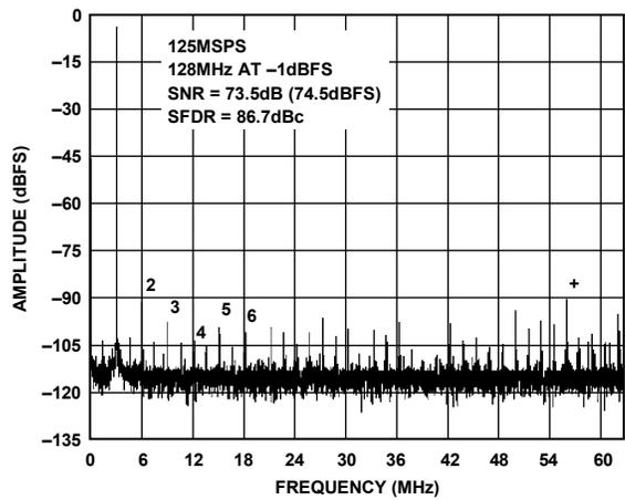
Figure 28. Single-Tone 16k FFT with  $f_{IN} = 128\text{ MHz}$ ,  $f_{SAMPLE} = 125\text{ MSPS}$ ,  $V_{REF} = 1.3\text{ V}$
