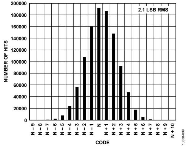
Figure 39. Input-Referred Noise Histogram,  $f_{SAMPLE} = 125$  MSPS,  $V_{REF} = 1.3$  V
