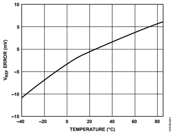
Figure 61. Typical  $V_{REF} = 1.3$  V Drift
