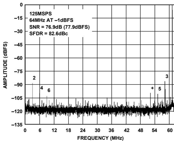
Figure 26. Single-Tone 16k FFT with  $f_{IN} = 64\text{ MHz}$ ,  $f_{SAMPLE} = 125\text{ MSPS}$ ,  $V_{REF} = 1.3\text{ V}$
