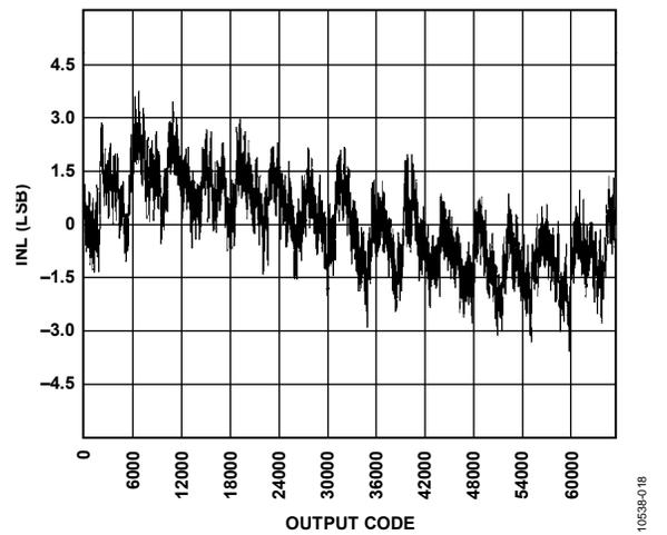
Figure 18. INL,  $f_{IN} = 9.7$  MHz,  $f_{SAMPLE} = 125$  MSPS,  $V_{REF} = 1.0$  V
