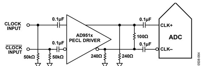
Figure 64. Differential PECL Sample Clock (Up to 1 GHz)
