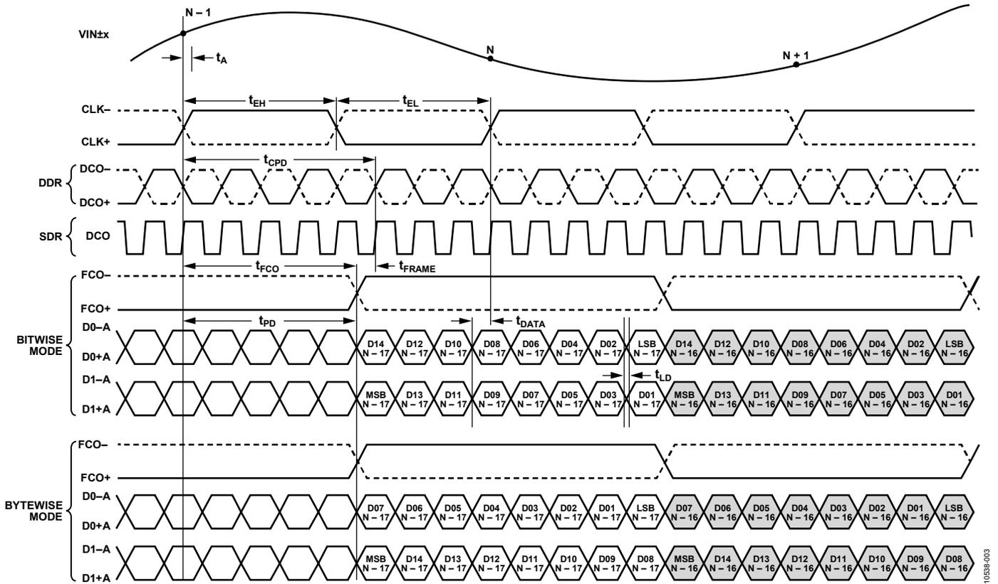
Figure 3. 16-Bit DDR/SDR, Two-Lane, 2x Frame Mode
