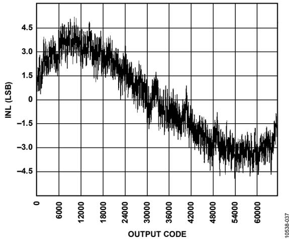
Figure 37. INL,  $f_{IN} = 9.7$  MHz,  $f_{SAMPLE} = 125$  MSPS,  $V_{REF} = 1.3$  V
