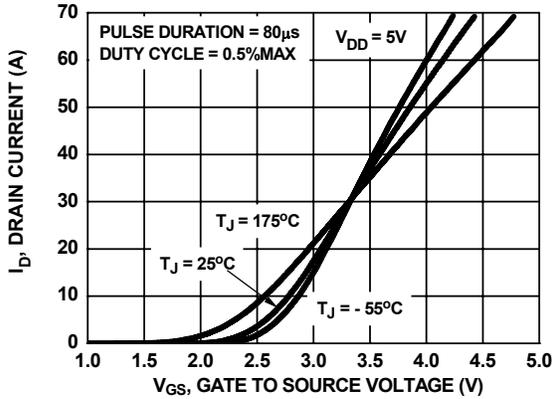
Figure 5. Transfer Characteristics
