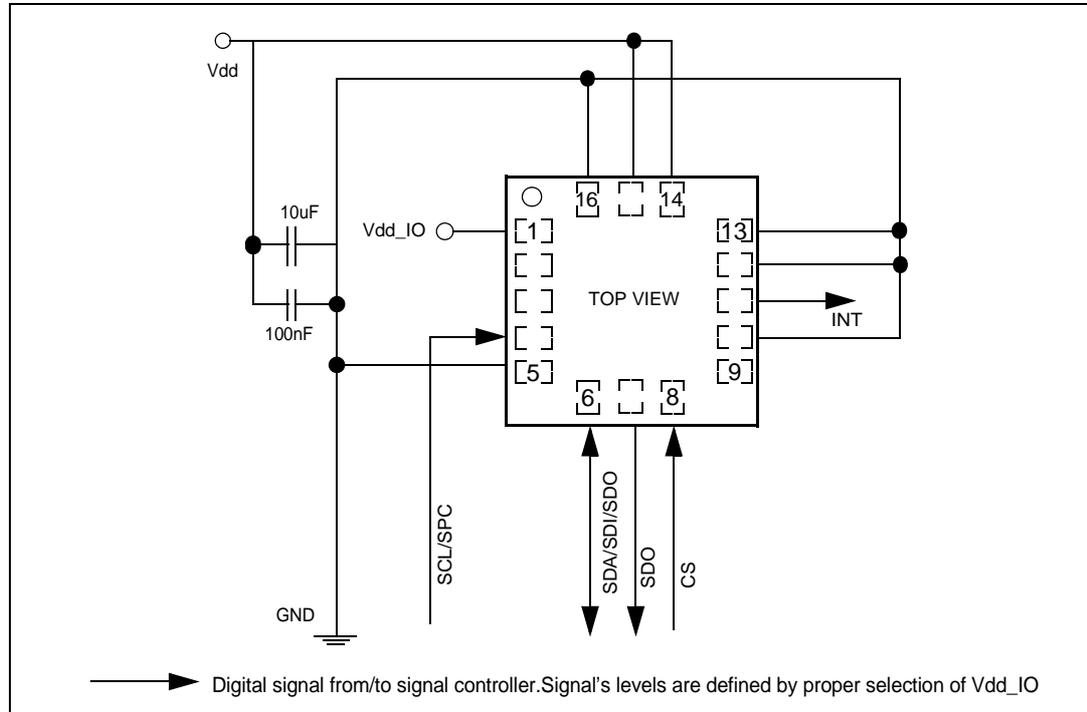
The device core is supplied through Vdd line while the I/O pads are supplied through Vdd\_IO line. Power supply decoupling capacitors (100 nF ceramic, 10  $\mu$ F Al) should be placed as near as possible to the pin 14 of the device (common design practice).
