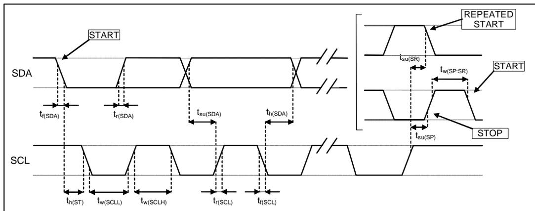
4. Measurement points are done at 0.2·Vdd\_IO and 0.8·Vdd\_IO, for both ports
