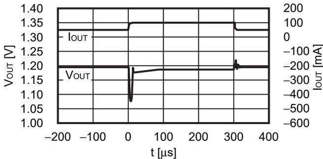
V<sub>IN</sub> = 2.2 V, C<sub>IN</sub> = C<sub>L</sub> = 1.0 μF, I<sub>OUT</sub> = 1 mA ↔ 150 mA
