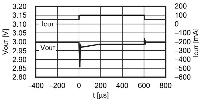
V<sub>IN</sub> = 4.0 V, C<sub>IN</sub> = C<sub>L</sub> = 1.0 μF, I<sub>OUT</sub> = 1 mA ↔ 150 mA
