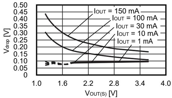
**Remark** In dashed line areas, the reverse current protection mode and the normal operation mode are repeated.
