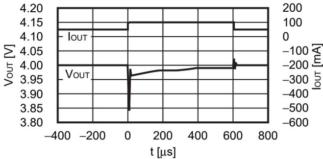
$V_{IN} = 5.0\text{ V}$ ,  $C_{IN} = C_L = 1.0\ \mu\text{F}$ ,  $I_{OUT} = 1\text{ mA} \leftrightarrow 150\text{ mA}$
