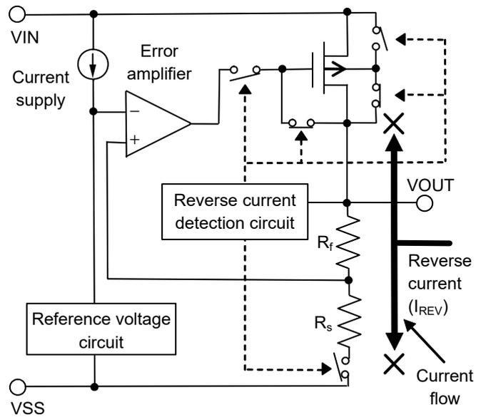
Figure 23 Reverse Current Protection Mode
