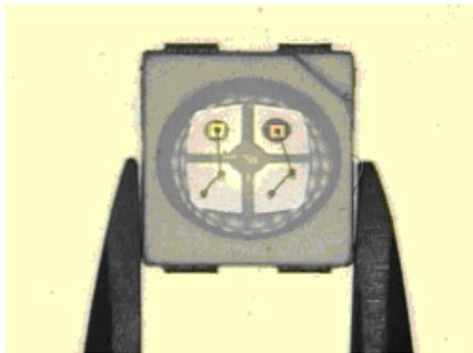
(3) When populating boards in SMT production, there are basically no restrictions regarding the form of the pick and place nozzle, except that mechanical pressure on the surface of the resin must be prevented.
