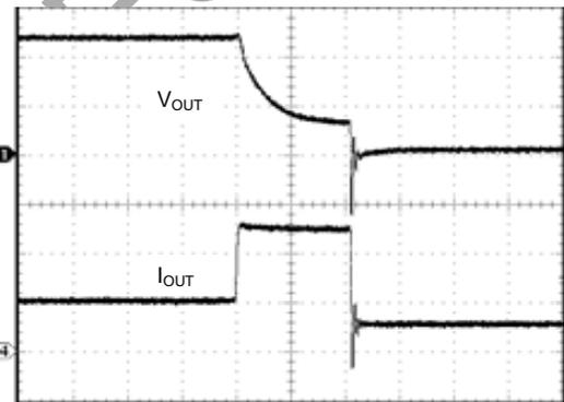
$C_{OUT} = 10\mu F$ ,  $C_{IN} = 10\mu F$ ,  $I_{OUT} = 2A$  to  $5.6A$
