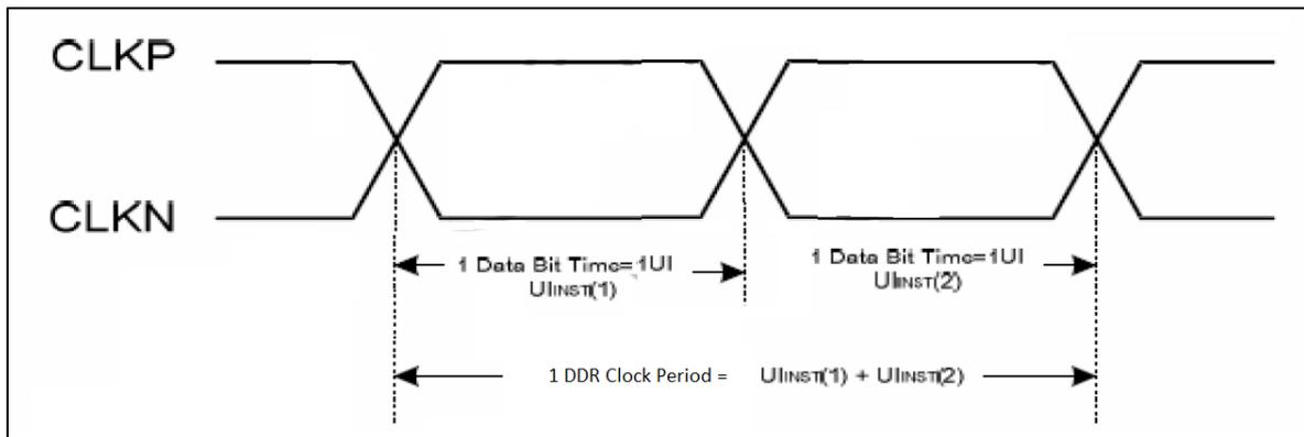
The same clock source is used to generate the DDR clock and launch the serial data. Since the clock and data signals propagate together over a channel of specified skew, the clock may be used directly to sample the data lines in the receiver. Such a system can accommodate large instantaneous variations in UI.
