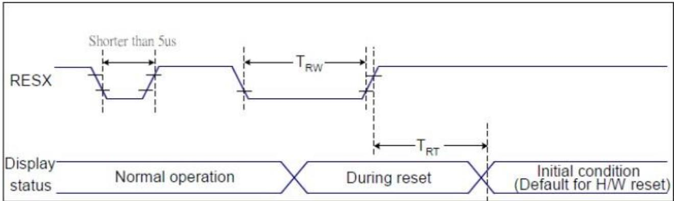
Figure 7 Reset Timing
