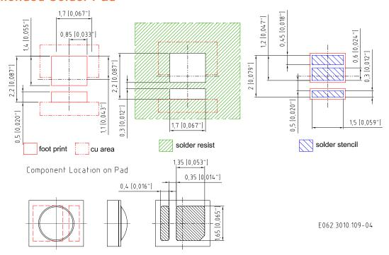
For superior solder joint connectivity results we recommend soldering under standard nitrogen atmosphere. Package not suitable for ultra sonic cleaning.
