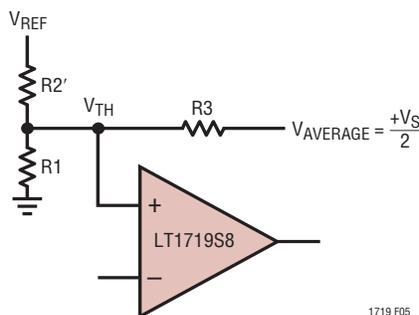
Figure 5. Model for Additional Hysteresis Calculations
