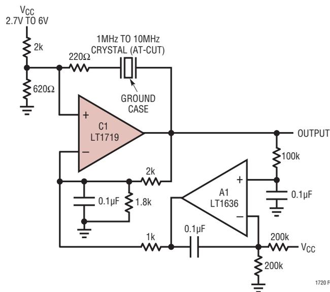
Figure 8. Crystal Oscillator with a Forced 50% Duty Cycle
