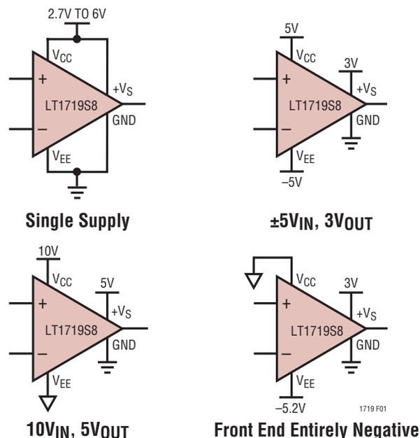
Figure 1. Variety of SO-8 Power Supply Configurations
