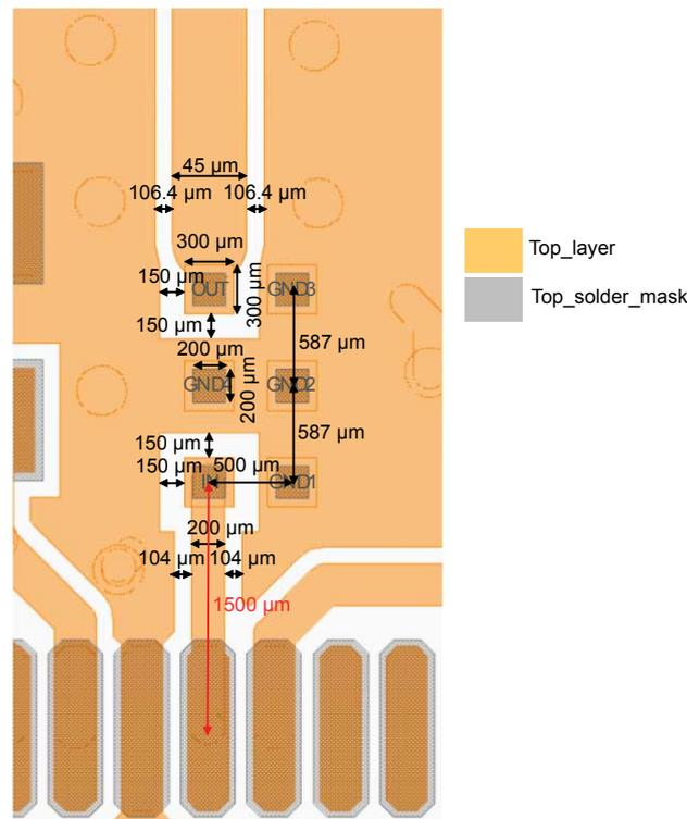
Transmission line between MLPF and antenna is dimensioned to 50 ohms characteristic impedance.
