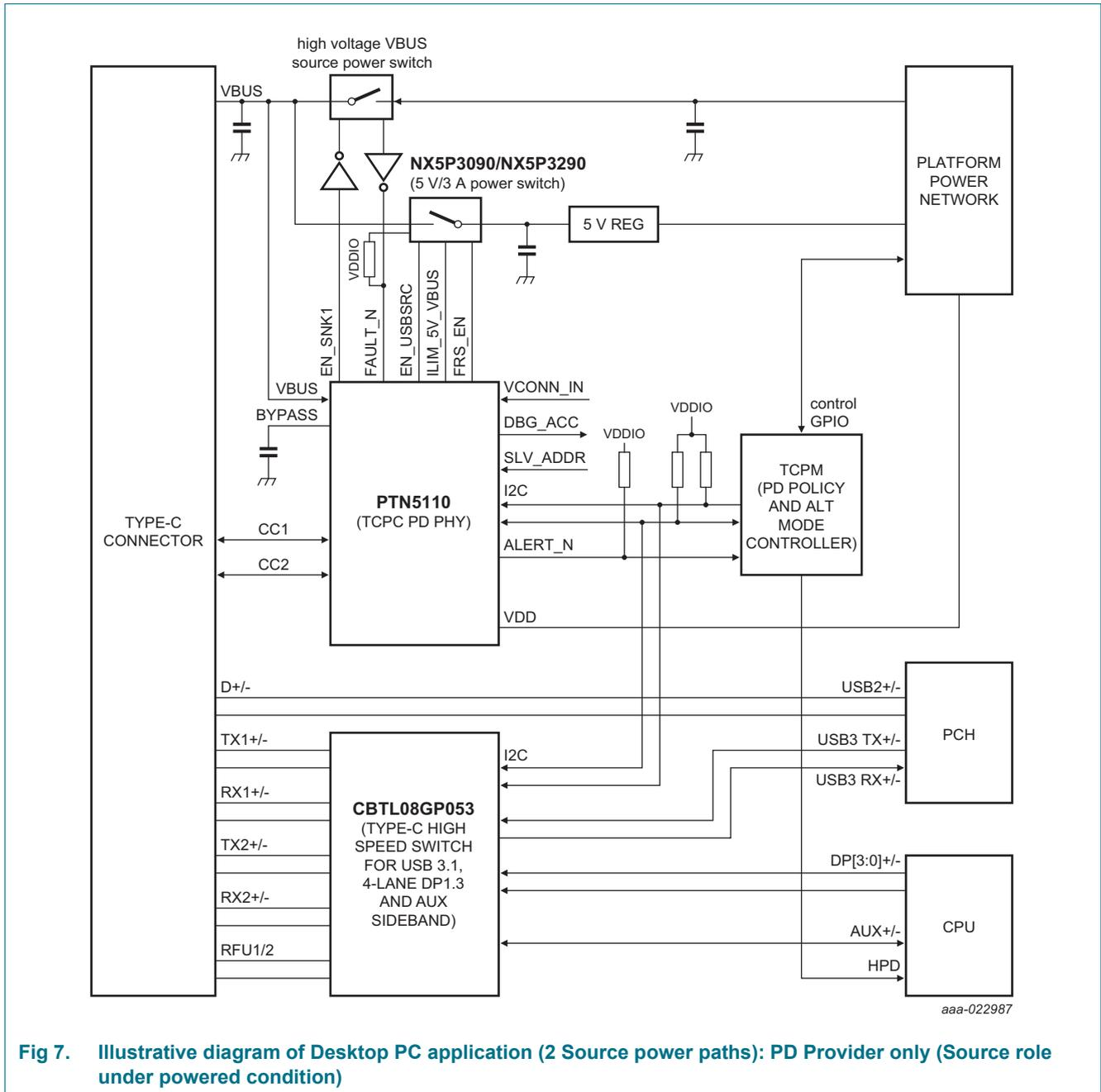
**Fig 7. Illustrative diagram of Desktop PC application (2 Source power paths): PD Provider only (Source role under powered condition)**
