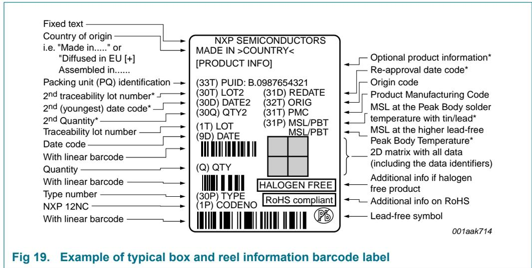
Fig 19. Example of typical box and reel information barcode label
