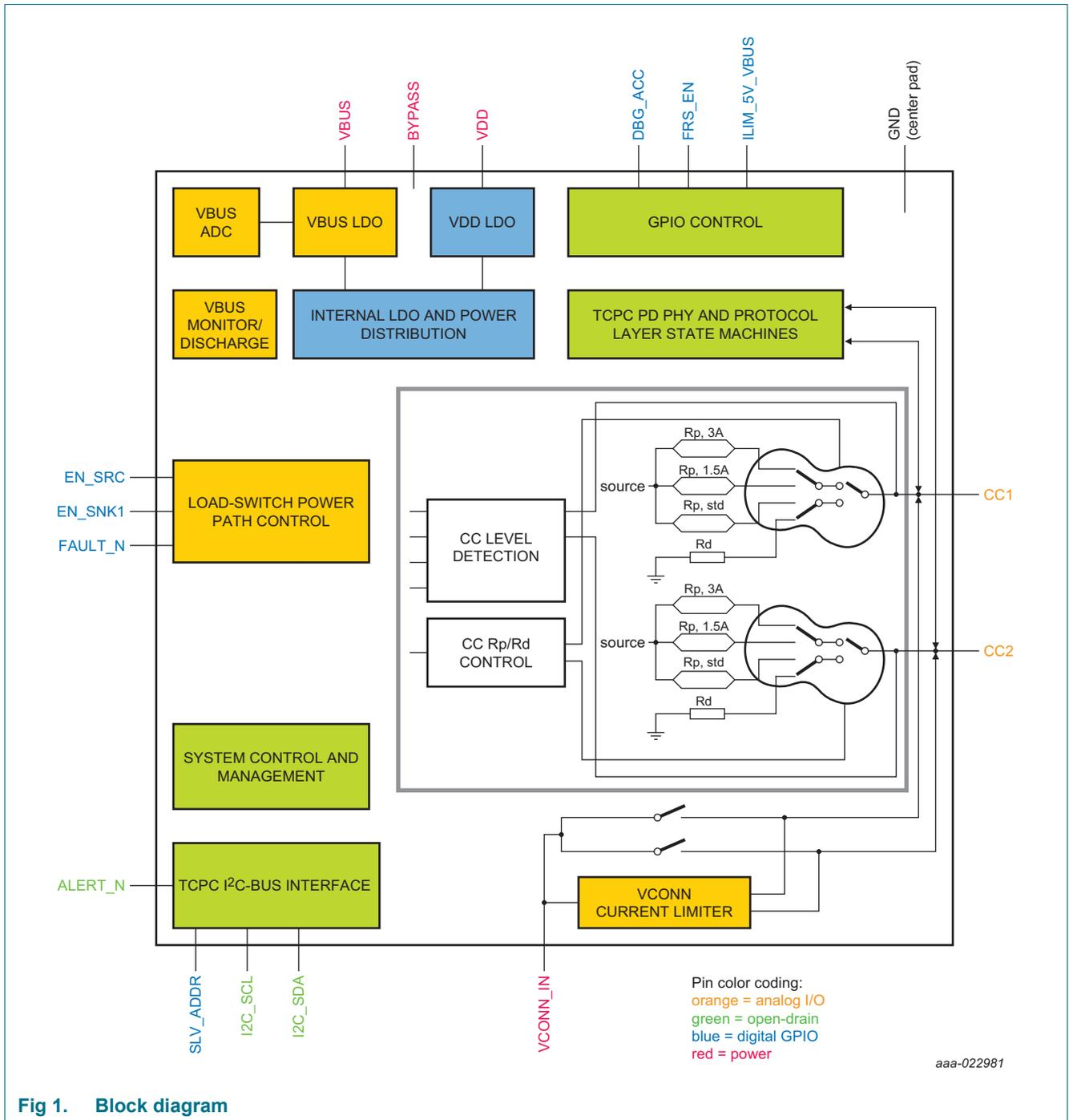
Fig 1. Block diagram
