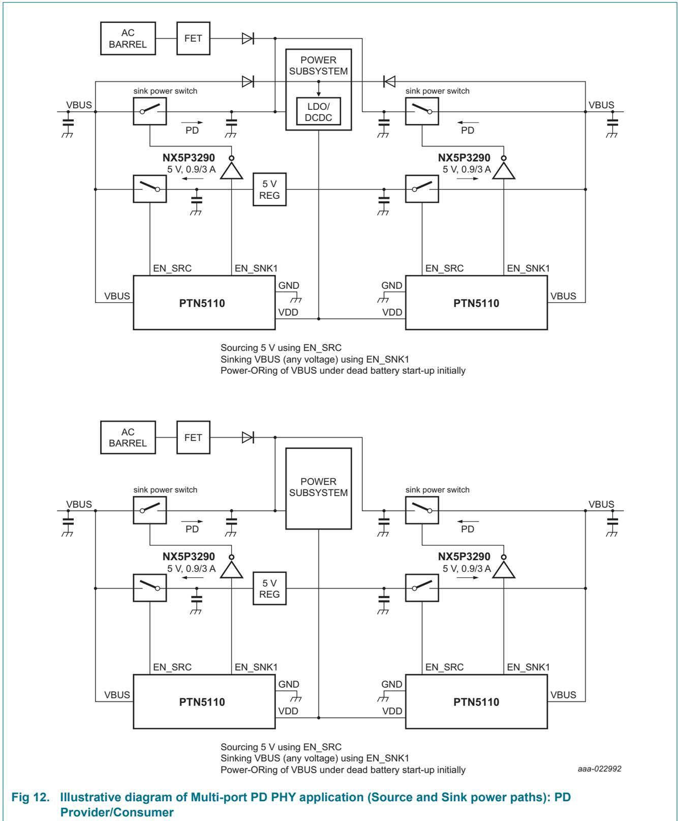
**Fig 12. Illustrative diagram of Multi-port PD PHY application (Source and Sink power paths): PD Provider/Consumer**
