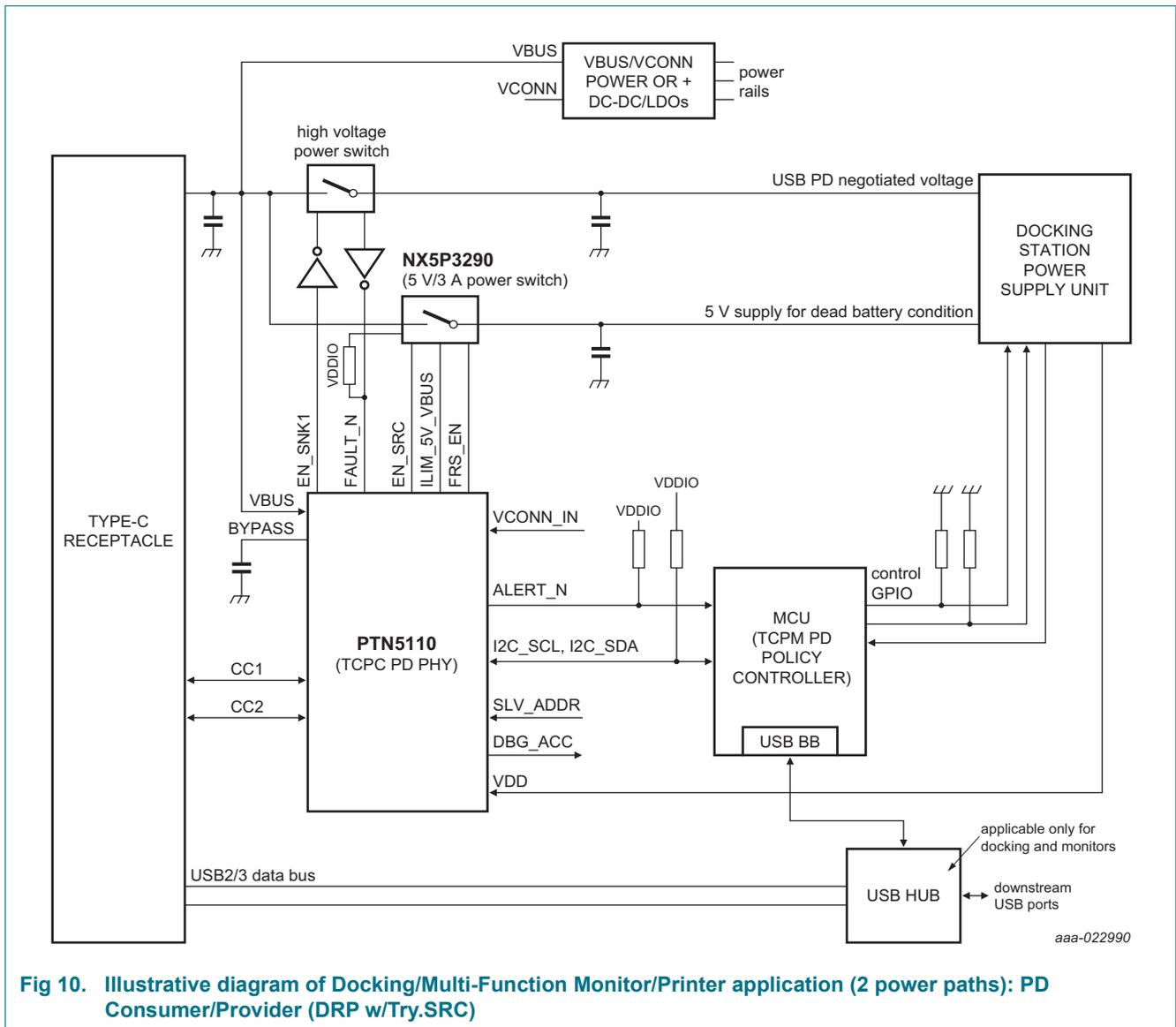
**Fig 10. Illustrative diagram of Docking/Multi-Function Monitor/Printer application (2 power paths): PD Consumer/Provider (DRP w/Try.SRC)**
