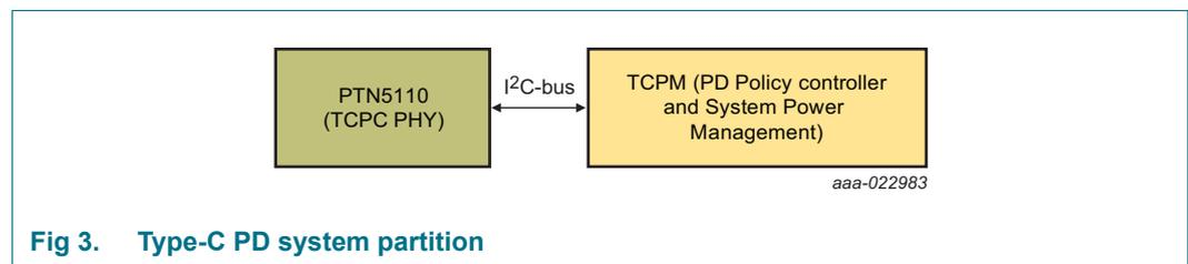
**Fig 3. Type-C PD system partition**
