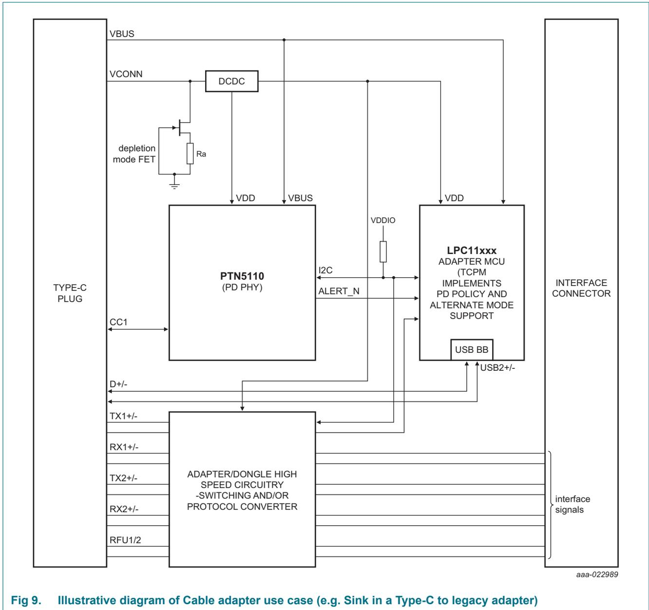
**Fig 9. Illustrative diagram of Cable adapter use case (e.g. Sink in a Type-C to legacy adapter)**
