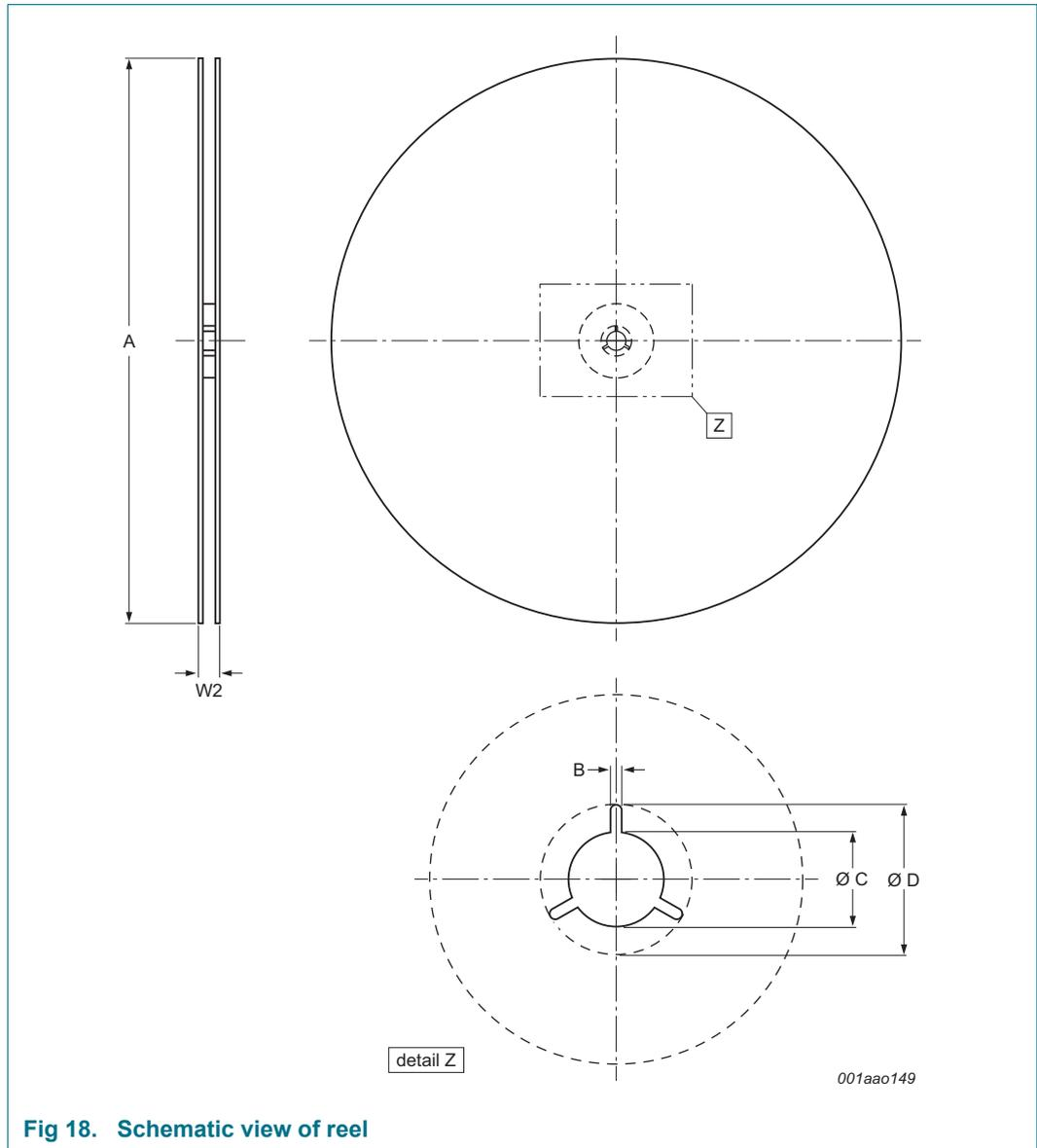
Fig 18. Schematic view of reel
