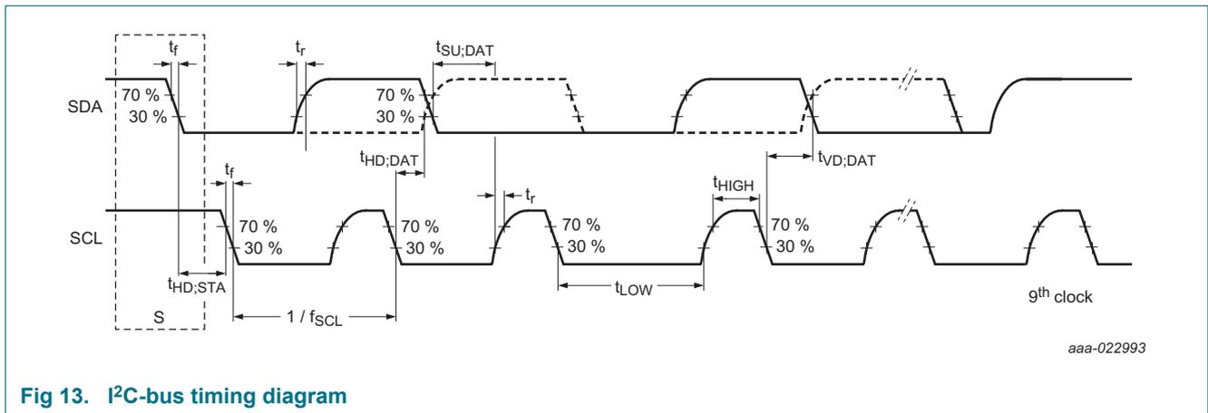
**Fig 13. I<sup>2</sup>C-bus timing diagram**
