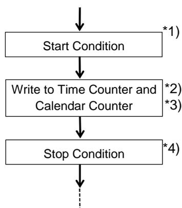
\*1) When writing to clock and calendar counters, do not insert Stop Condition until all times from second to year have been written to prevent error in writing time. (Detailed in "P.28 Data Transmission under Special Condition".
