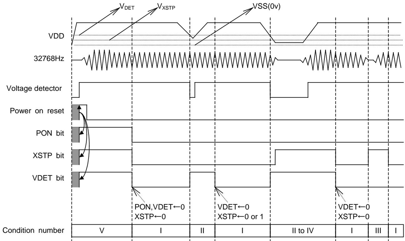
\*) The power on reset shown above is an internal signal and the signal is generated from right after the VDD turns on until the oscillation of quartz crystal unit starts. While the term of the power-on reset signal is out, or the time until the oscillation of quartz crystal unit starts, approximately 0.1s to 1.0s, access of I2C bus is impossible.
