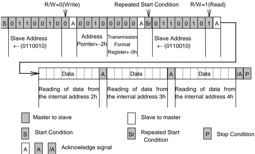
The second method to reading data from the internal register is to start reading immediately after writing to the Internal Address Pointer and the Transmission Format Register. Although this method is not based on I<sup>2</sup>C-Bus standard in a strict sense it still effective to shorten read time to ease load to the master. Set 4h or 5h to the transmission format register when this method used.
