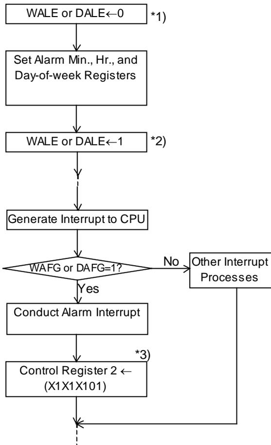
\*1) This step is intended to once disable the alarm interrupt circuit by setting the WALE or DALE bits to 0 in anticipation of the coincidental occurrence of a match between current time and preset alarm time in the process of setting the alarm interrupt function.
