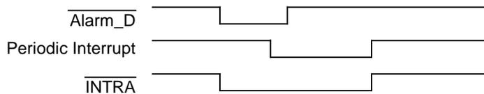
In this event, which type of interrupt signal is output from the  $\overline{\text{INTRA}}$  (R2221x= $\overline{\text{INTR}}$ ) pin can be confirmed by reading the DAFG, and CTFG bit settings in the Control Register 2.
