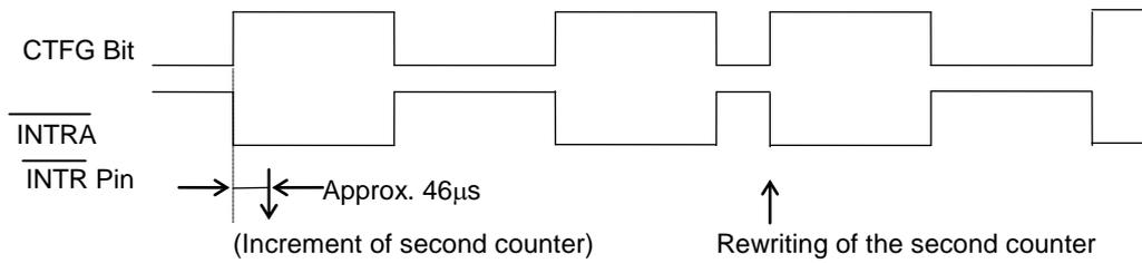
In the pulse mode, the increment of the second counter is delayed by approximately 46 µs from the falling edge of clock pulses. Consequently, time readings immediately after the falling edge of clock pulses may appear to lag behind the time counts of the real-time clocks by approximately 1 second. Rewriting the second counter will reset the other time counters of less than 1 second, driving the  $\overline{\text{INTRA}}$  ( $\overline{\text{INTR}}$ ) pin low.
