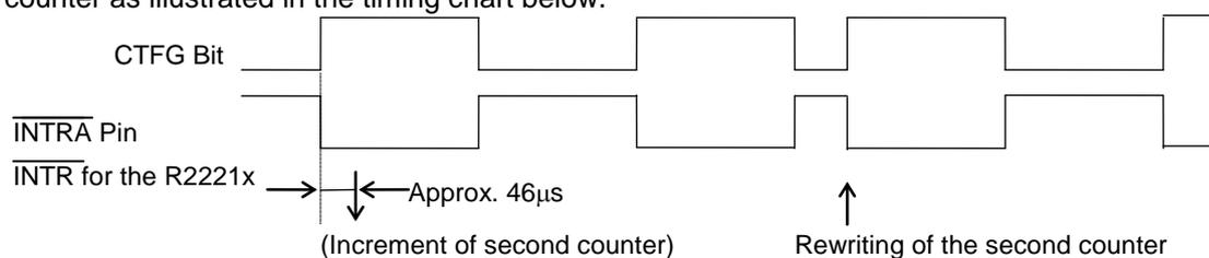
In the pulse mode, the increment of the second counter is delayed by approximately 46 µs from the falling edge of clock pulses. Consequently, time readings immediately after the falling edge of clock pulses may appear to lag behind the time counts of the real-time clocks by approximately 1 second. Rewriting the second counter will reset the other time counters of less than 1 second, driving the  $\overline{\text{INTRA}}$  ( $\overline{\text{INTR}}$ ) pin low.
