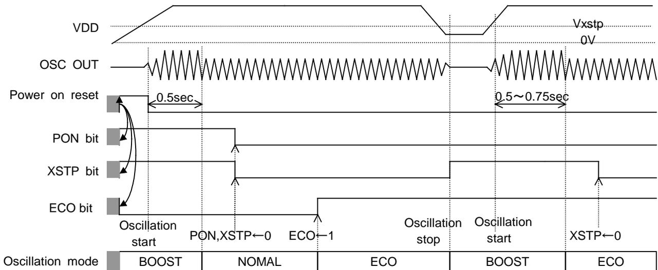
\*) The power on reset shown above is an internal signal and the signal is generated from right after the VDD turns on until the oscillation of quartz crystal unit starts. While the term of the power-on reset signal is out, or the time until the oscillation of quartz crystal unit starts, approximately 0.1s to 1.0s, access of I2C bus is impossible.
