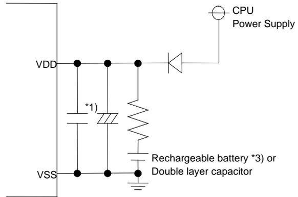
\*1) Set bypass capacitors as close as possible to the IC, use a capacitor for high frequency and another capacitor for low frequency in parallel.
