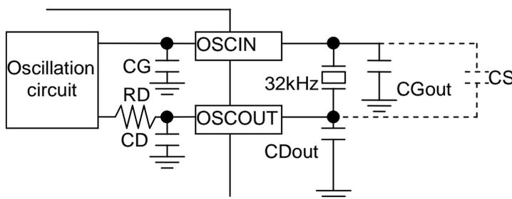
\*1) The CGOUT or/and CDOUT should have a capacitance ranging from 0 to 6 pF. (Including parasitic capacitance of the printed circuit board)
