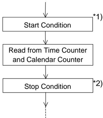
\*1) When reading to clock and calendar counters, do not insert Stop Condition until all times from second to year have been written to prevent error in writing time. (Detailed in "P.28 Data Transmission under Special Condition").
