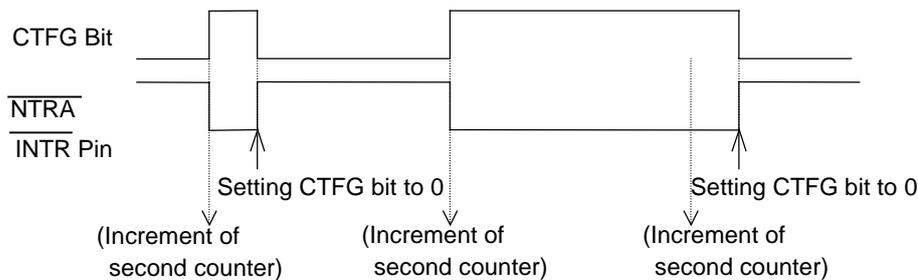
\*1), \*2) When the oscillation adjustment circuit is used, the interrupt cycle will fluctuate once per 20sec. as follows:
