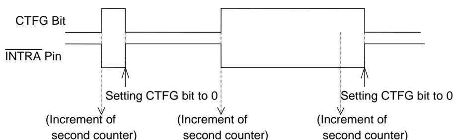
At the level mode, the moment right after writing CT2-CT0,  $\overline{\text{INTRA}}$  ( $\overline{\text{INTR}}$ ) pin becomes "L" in very short moment. In such a case, ignore it or confirm it by CTFG bit.
