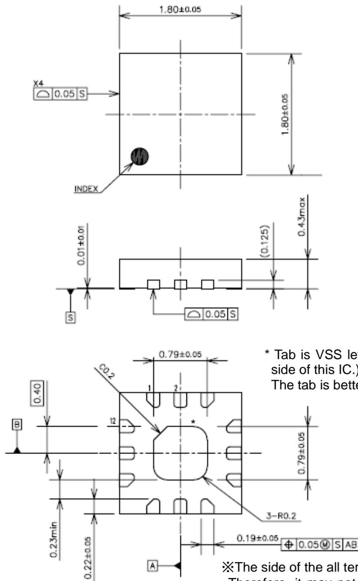
\* Tab is VSS level. (They are connected to the reverse side of this IC.)
