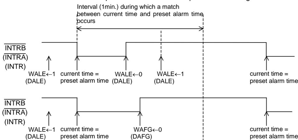
After setting WALE(DALW) to 0, Alarm registers is set to current time, and WALE(DALE) is set to 1,  $\overline{\text{INTRB}}$  (  $\overline{\text{INTRA}}$  ) will be not driven to "L" immediately,  $\overline{\text{INTRB}}$  (  $\overline{\text{INTRA}}$  ,  $\overline{\text{INTR}}$  ) will be driven to "L" at next alarm setting time.
