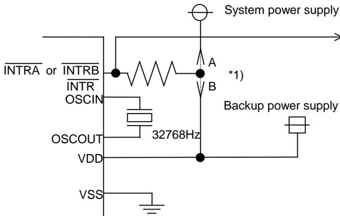
\*1) Depending on whether the  $\overline{\text{INTRA}}$  or  $\overline{\text{INTRB}}$  (R2223x),  $\overline{\text{INTR}}$  (R2221x) pin is used during battery backup, it should be connected to a pull-up resistor at the following different positions:
