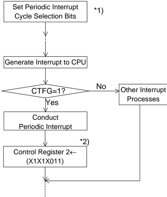
\*1) This step is intended to select the level mode as a waveform mode for the periodic interrupt function.
