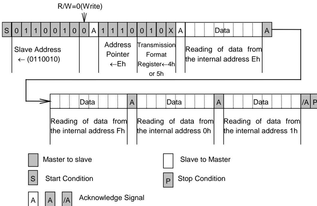
The third method to reading data from the internal register is to start reading immediately after writing to the Slave Address and R/W bit. Since the Internal Address Pointer is set to Fh by default as described in the first method, this method is only effective when reading is started from the Internal Address Fh.
