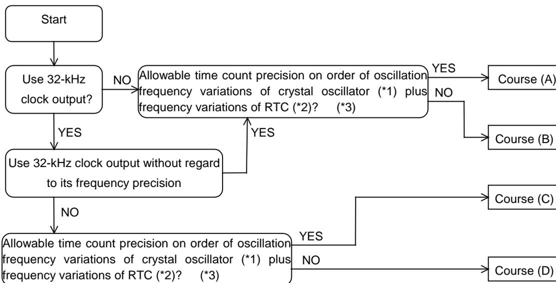
\* 1) Generally, quartz crystal units for commercial use are classified in terms of their center frequency depending on their load capacitance (CL) and further divided into ranks on the order of ±10, ±20, and ±50ppm depending on the degree of their oscillation frequency variations.
