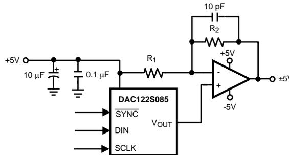
**Figure 35. Bipolar Operation**
