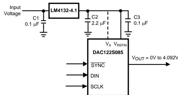
**Figure 31. The LM4130 as a power supply**
