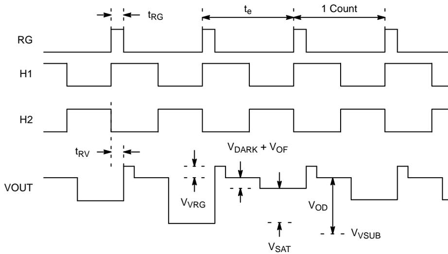
Figure 15. Pixel Timing
