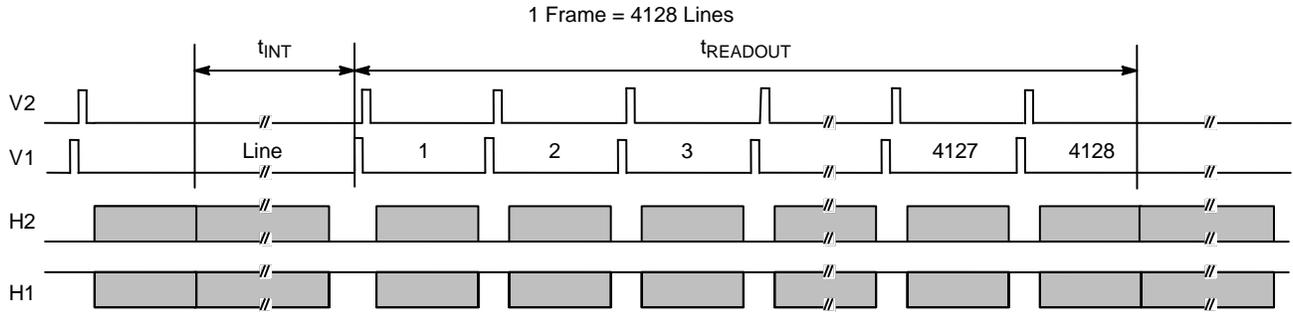
Figure 12. Frame Timing
