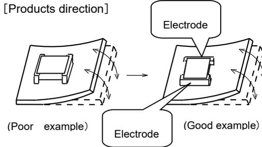
The electrode part of the products should be located like the picture to the mechanical stress.
