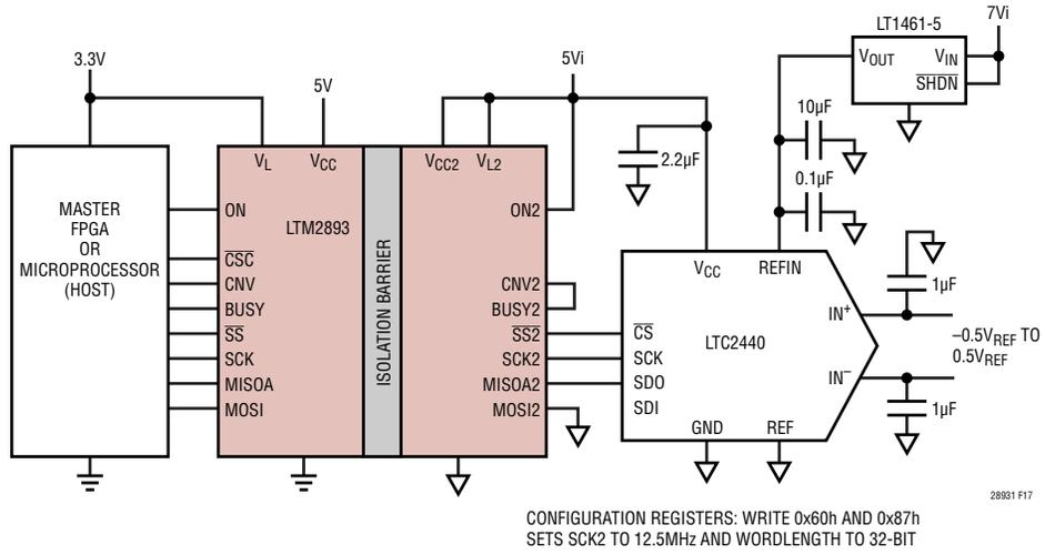
Figure 17. LTM2893 with LTC2440 Delta Sigma ADC
