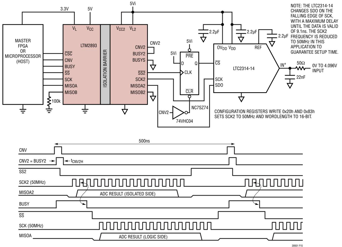
**Figure 15. Isolated 2Msps LTC2314-14 0V to 4.096V Input Range, ADC Without a CNV or BUSY, LTC2314 CS Is Synchronized to Low Jitter CNV2**
