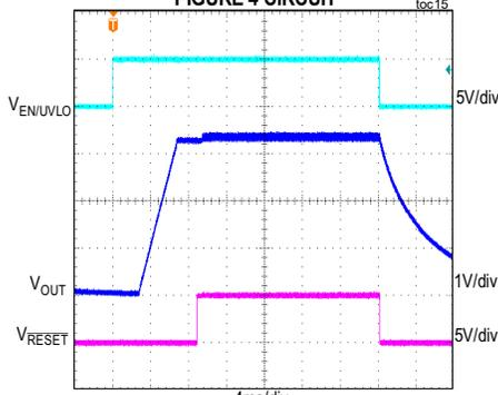
CONDITION:  $\overline{RESET}$  IS PULLED UP TO  $V_{CC}$  WITH A 10kΩ RESISTOR
