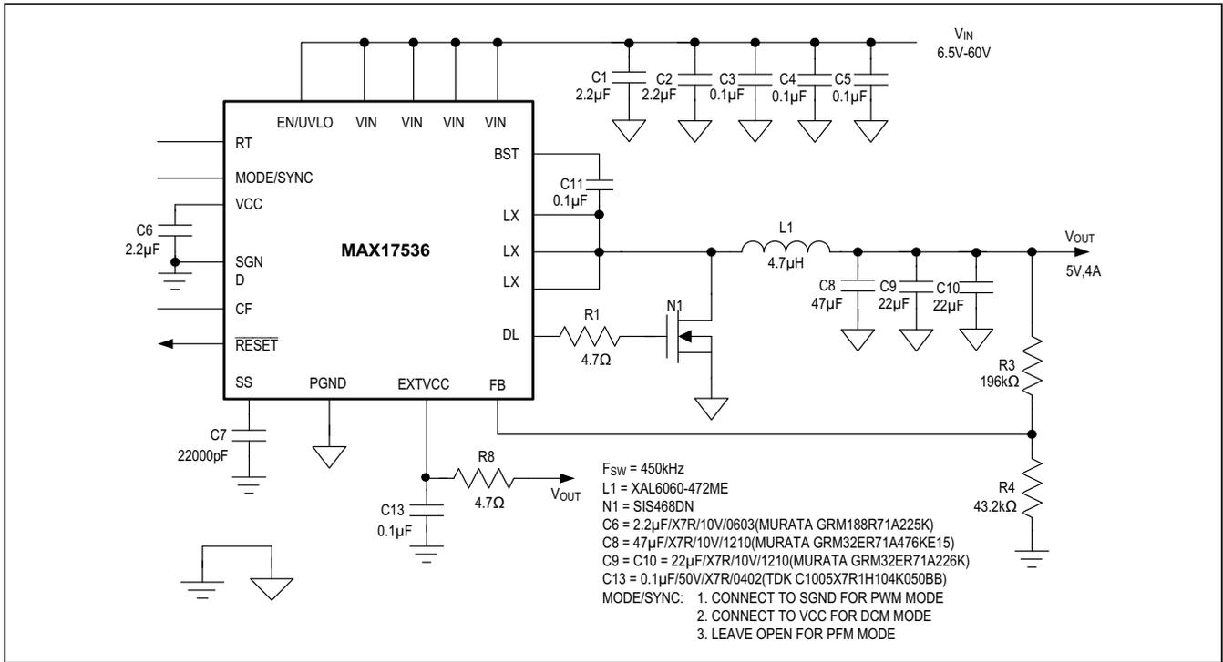
Figure 3. Typical Application Circuit for 5V Output
