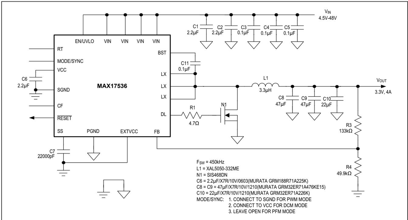
Figure 4. Typical Application Circuit for 3.3V Output
