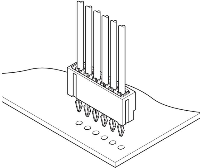
Measuring 2.0 mm in pitch, 6.0 mm in mounting height, and 3.25 mm in thickness, this board-in connector meets the needs for high-density mounting on printed circuit boards efficiently and economically. The connector is ideal for VCRs, car stereo systems, audio products and many other consumer oriented electronic products.
