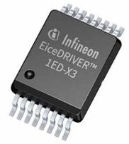
The EiceDRIVER™ Enhanced X3 Digital family (1ED38xx) provides I2C configurability for DESAT, soft-off, UVLO, Miller clamp, two level turn off (TLTO), and Fault function to simplify the design of highly reliable systems. All adjustments are done from the input side via the I2C interface (pin SDA and SCL). 1ED38xx offers up to 9 A current, in DSO-16 300 mil fine pitch package.
