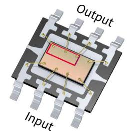
Using this mixed-signal HVIC technology, both high-voltage level-shifting circuits and low-voltage analog and digital circuits can be implemented. This is done with the ability to place high-voltage circuitry (in a 'well' formed by polysilicon rings).
