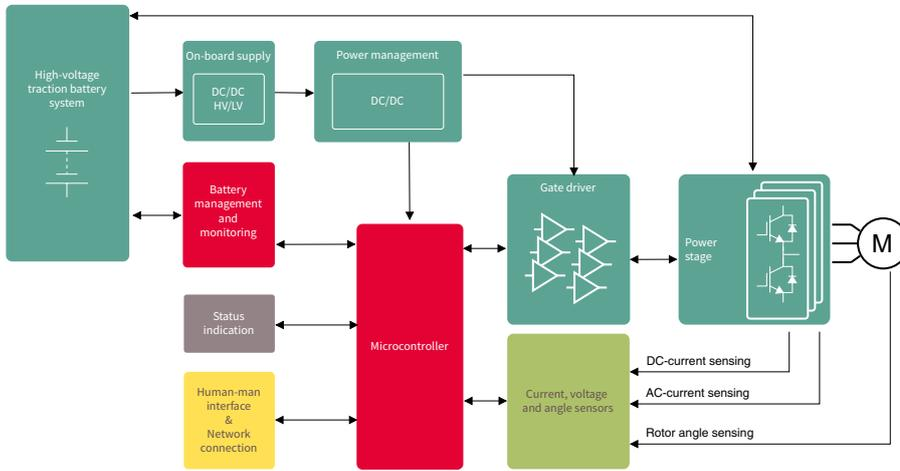
Compactness, reliability and efficiency. These factors, along with safety and robustness, are what distinguish successful powertrain inverter for truck and agricultural vehicle designs from the rest. A scalable system level solution that reduces the time to market and the total cost of ownership is key.
