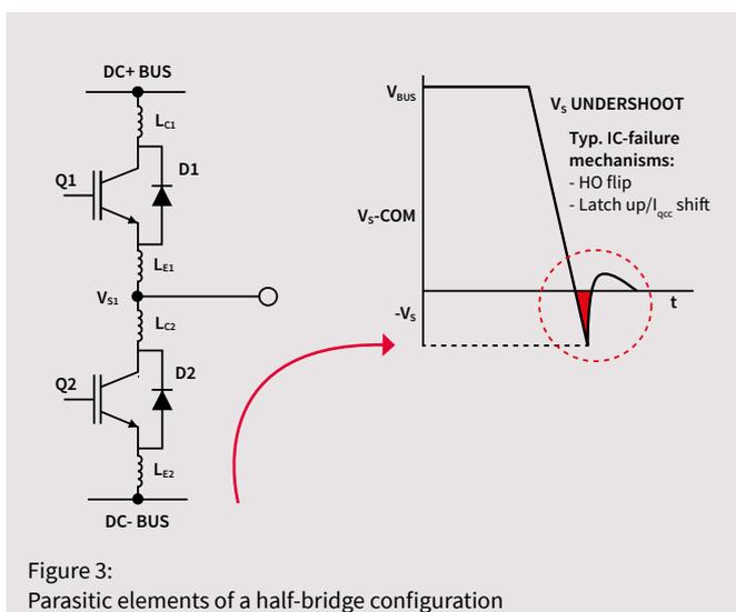
Figure 3: Parasitic elements of a half-bridge configuration
