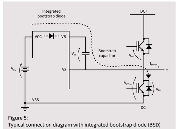
Figure 5: Typical connection diagram with integrated bootstrap diode (BSD)
