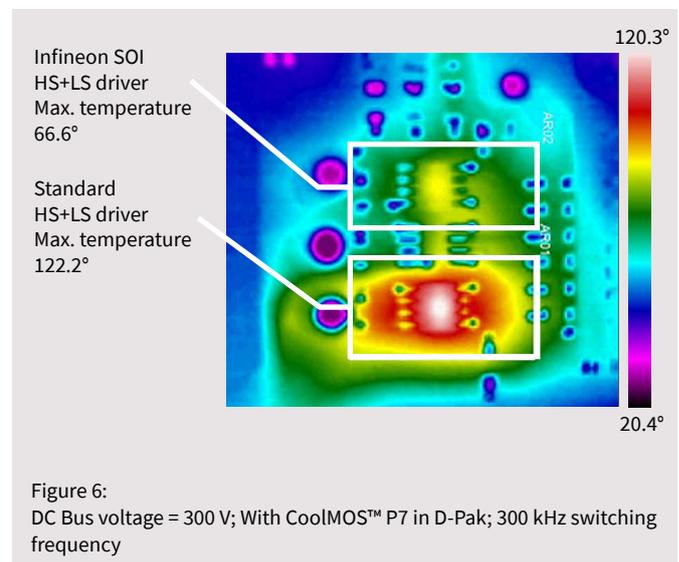
Figure 6: DC Bus voltage = 300 V; With CoolMOS™ P7 in D-Pak; 300 kHz switching frequency
