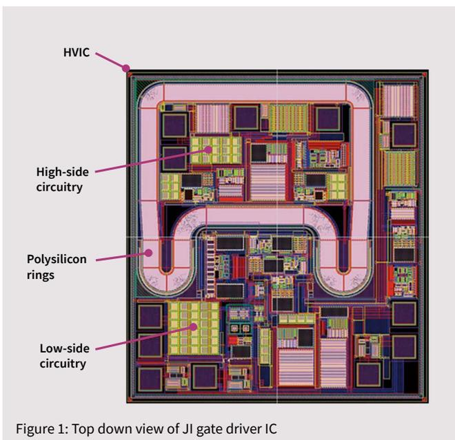
Figure 1: Top down view of JI gate driver IC
