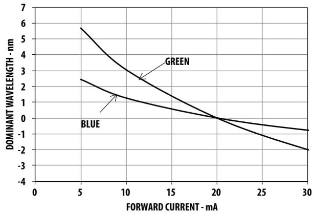
Figure 5. Dominant Wavelength Shift vs Forward Current
