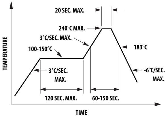
a. Reflow soldering must not be done more than two times. Do observe necessary precautions for handling a moisture-sensitive device, as stated in the following section.
