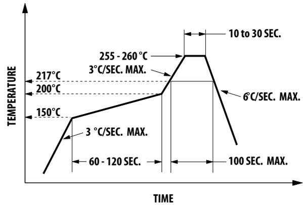
c. Do not apply any pressure or force on the LED during reflow and after reflow when the LED is still hot.
