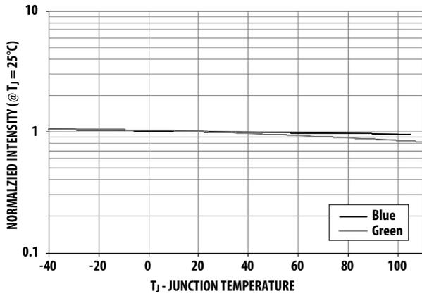
Figure 7. Relative Intensity Shift vs Junction Temperature
