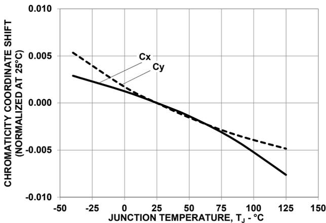
**Figure 13: Chromaticity Coordinate Shift vs. Junction Temperature – 6500K**
