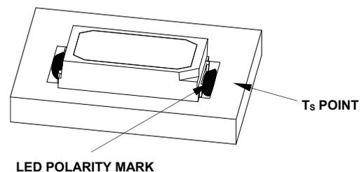
$T_S$  can be easily measured by mounting a thermocouple on the soldering joint as shown in preceding figure, while  $R_{\theta J-S}$  is provided in the data sheet. Verify the  $T_S$  of the LED in the final product to ensure that the LEDs are operating within all maximum ratings stated in the data sheet.
