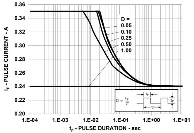
**Figure 17: Pulse Handling Capability at  $T_s = 100^{\circ}C$**
