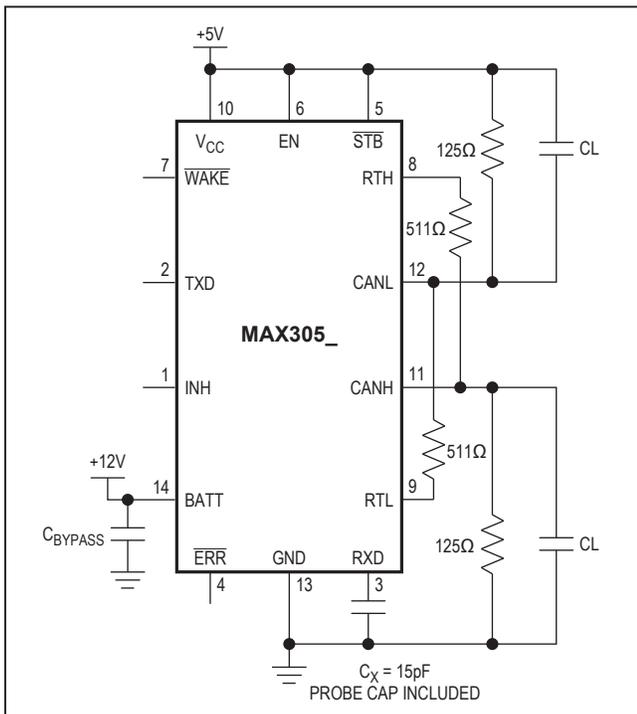
Figure 3. Test Circuit for Typical Operating Characteristics
