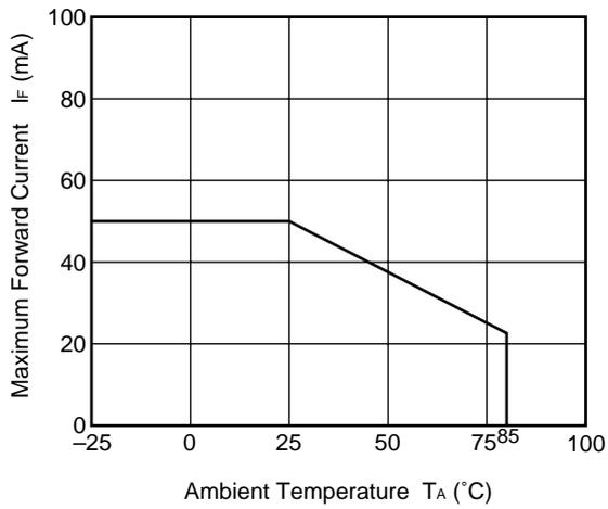
MAXIMUM LOAD CURRENT vs. AMBIENT TEMPERATURE
