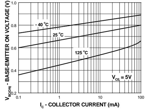
Figure 4. Base-Emitter On Voltage vs. Collector Current
