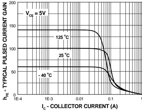
Figure 1. Typical Pulsed Current Gain vs. Collector Current
