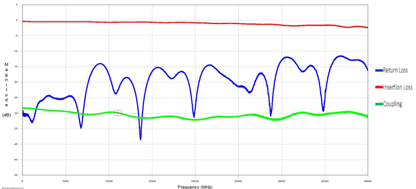
\*Typical measured performance mounted on RO4350B test board at 25°C.
