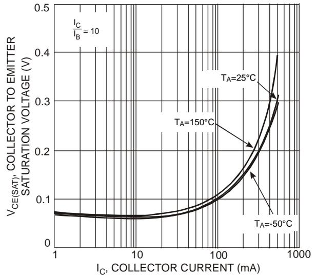
Fig. 5 Collector Emitter Saturation Voltage vs. Collector Current
