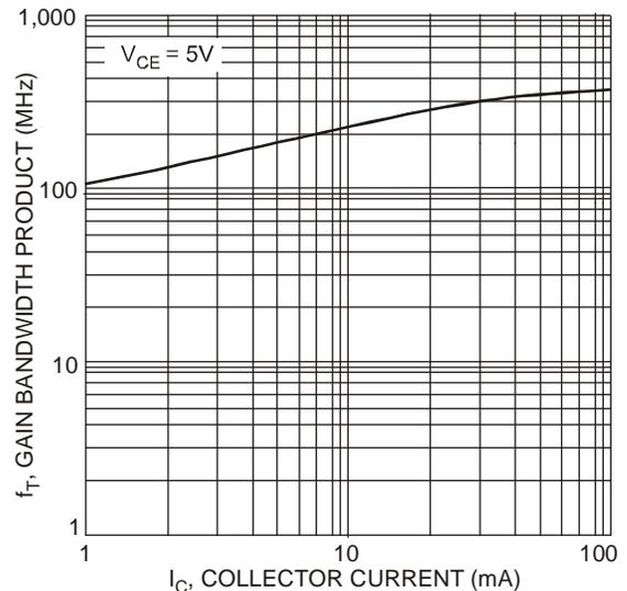
Fig. 7 Gain Bandwidth Product vs. Collector Current
