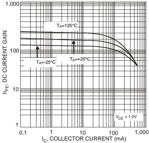
Fig. 2 Typical DC Current Gain vs. Collector Current
