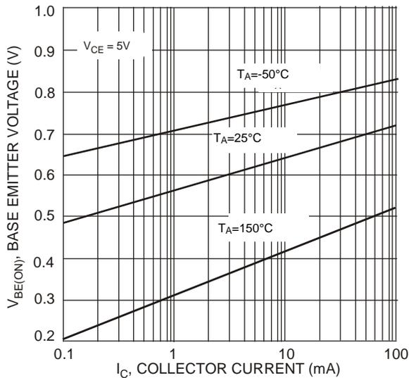
Fig. 6 Base Emitter Voltage vs. Collector Current
