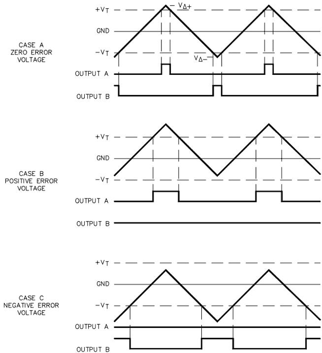
Figure 3 - Pulse Width Modulation with No Deadband
