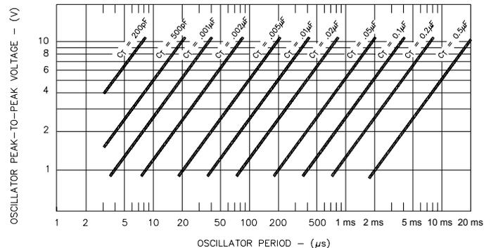
Figure 2 · SG1731 Oscillator Period VS.  $V_{\text{OSC}}$  and  $C_T$
