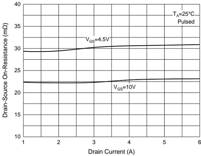
Fig. 4 -  $R_{DS(ON)} - V_{GS}$
