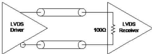
**Figure 6. LVDS to LVDS Connection, Internal 100ohm Resistor**
