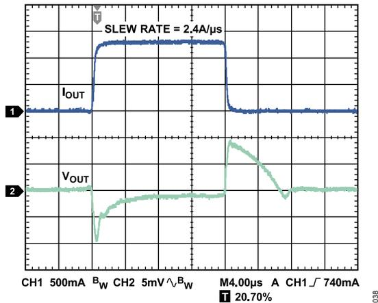
Figure 35. Load Transient Response,  $I_{LOAD} = 100 \text{ mA}$  to  $1.2 \text{ A}$ ,  $V_{OUT} = 1.8 \text{ V}$ ,  $V_{IN} = 2.5 \text{ V}$ ,  $C_{OUT} = 22 \mu\text{F}$ , Channel 1 =  $I_{OUT}$ , Channel 2 =  $V_{OUT}$
