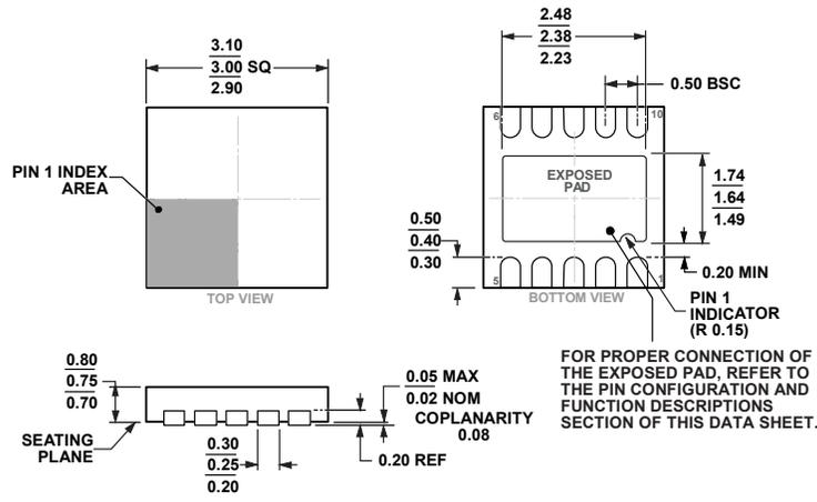
Figure 63. 10-Lead Lead Frame Chip Scale Package [LFCSP]
