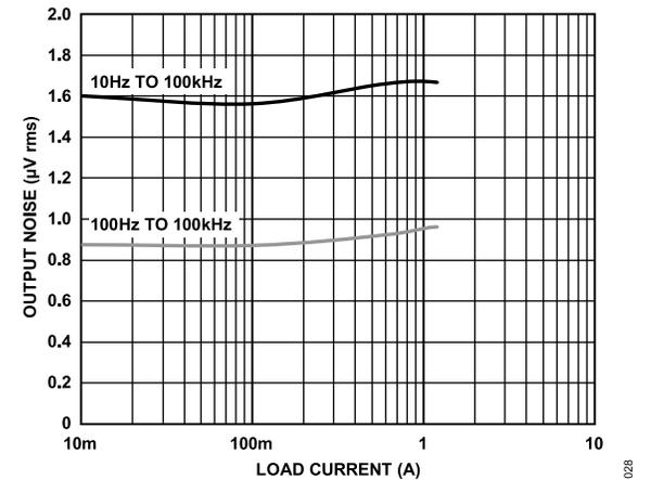
Figure 27. RMS Output Noise vs. Load Current
