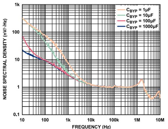
Figure 44. Noise Spectral Density vs. Frequency at Various  $C_{BYP}$  Values
