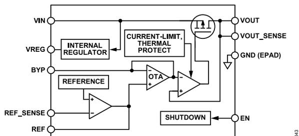
Figure 40. Simplified Internal Block Diagram
