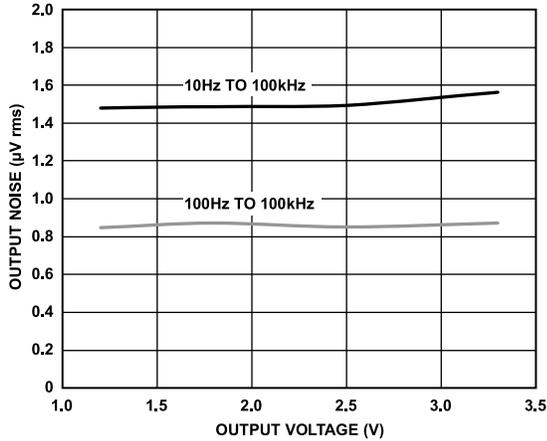
Figure 28. RMS Output Noise vs. Output Voltage
