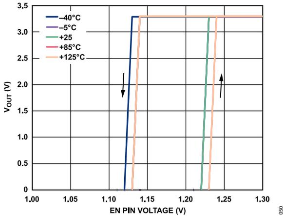
Figure 47. Typical  $V_{OUT}$  Response to EN Pin Operation
