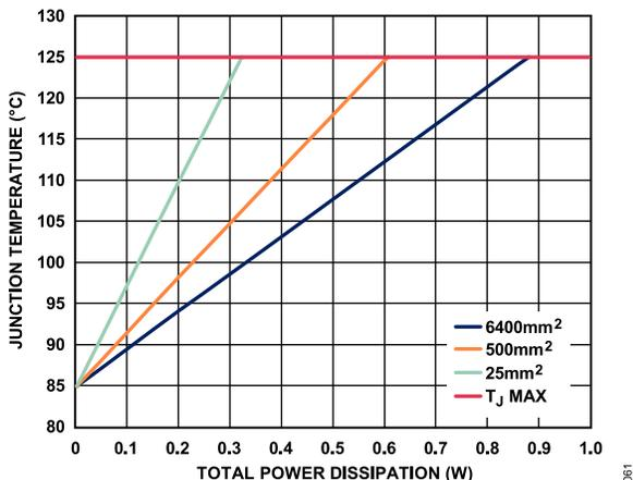
Figure 58. Junction Temperature vs. Total Power Dissipation for the 8-Lead SOIC,  $T_A = 85^\circ\text{C}$
