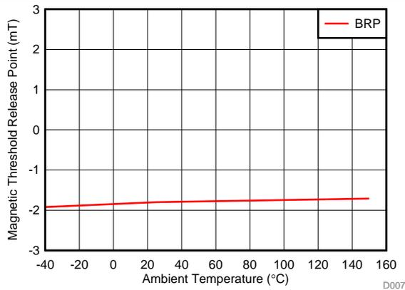
Figure 7.  $B_{RP}$  Threshold vs Temperature (DRV5015A2, DRV5015A3)
