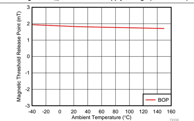
Figure 6.  $B_{OP}$  Threshold vs Temperature (DRV5015A2, DRV5015A3)
