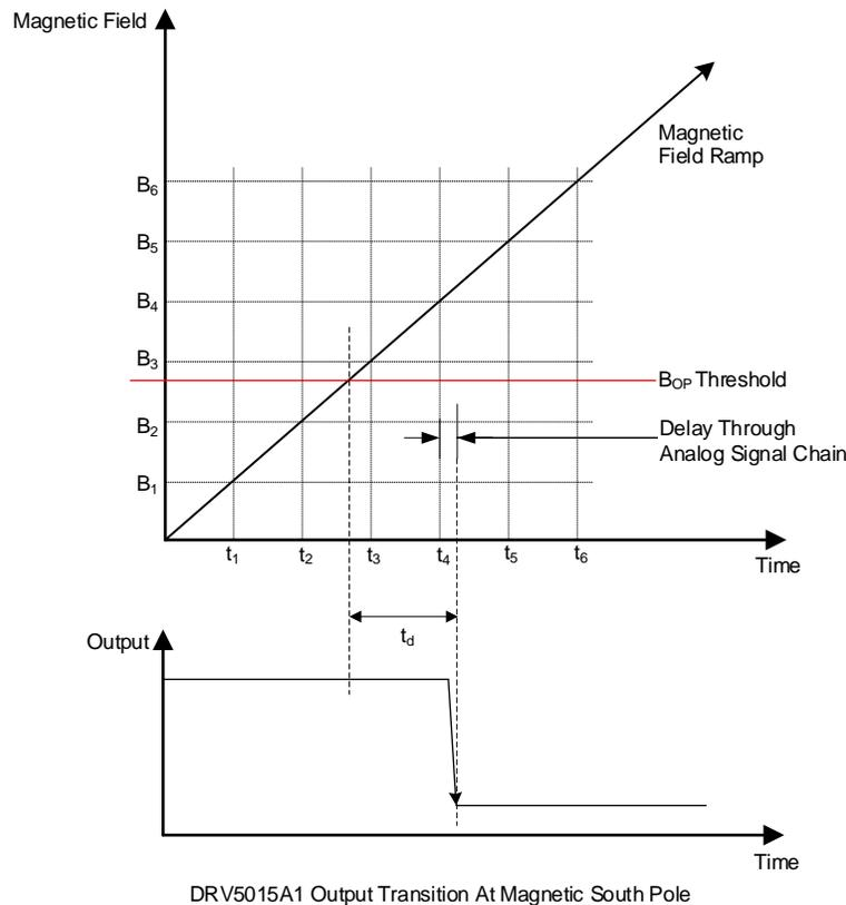
**Figure 17. Propagation Delay**
