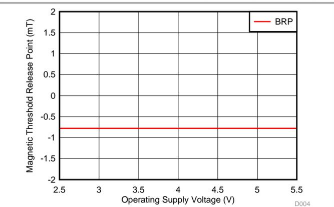
Figure 4.  $B_{RP}$  Threshold vs Supply Voltage (DRV5015A1)
