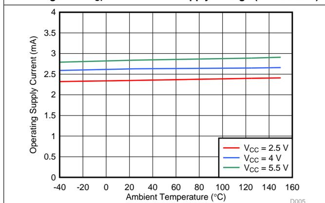
Figure 5.  $I_{CC}$  vs Temperature (DRV5015A1)
