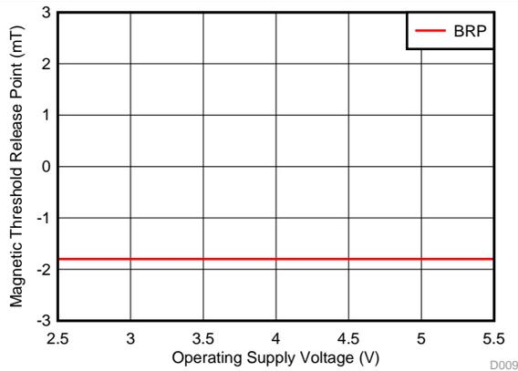
Figure 9.  $B_{RP}$  Threshold vs Supply Voltage (DRV5015A2, DRV5015A3)
