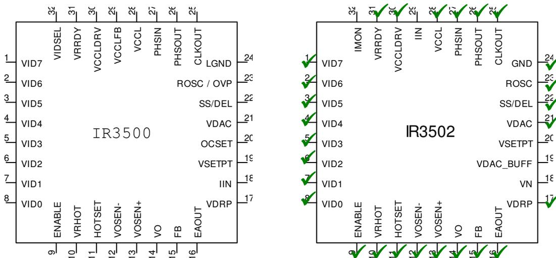
Figure 1 – PIN difference between IR3500 and IR3502
