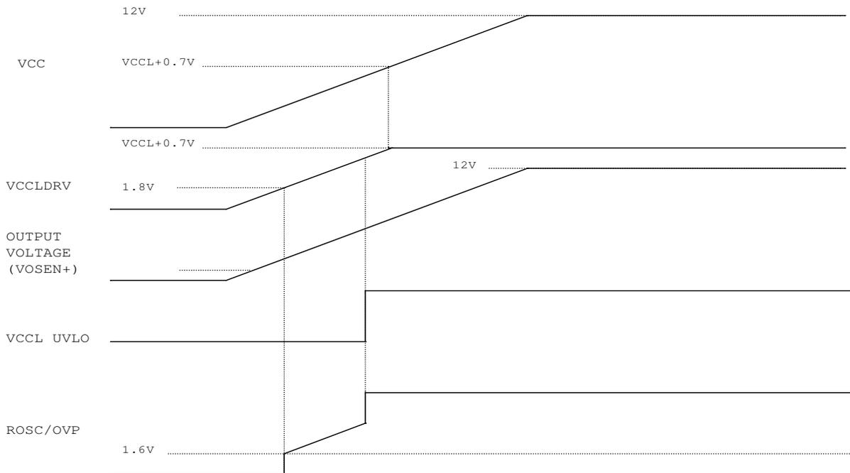
Figure 14 Over-voltage protection during power-up.
