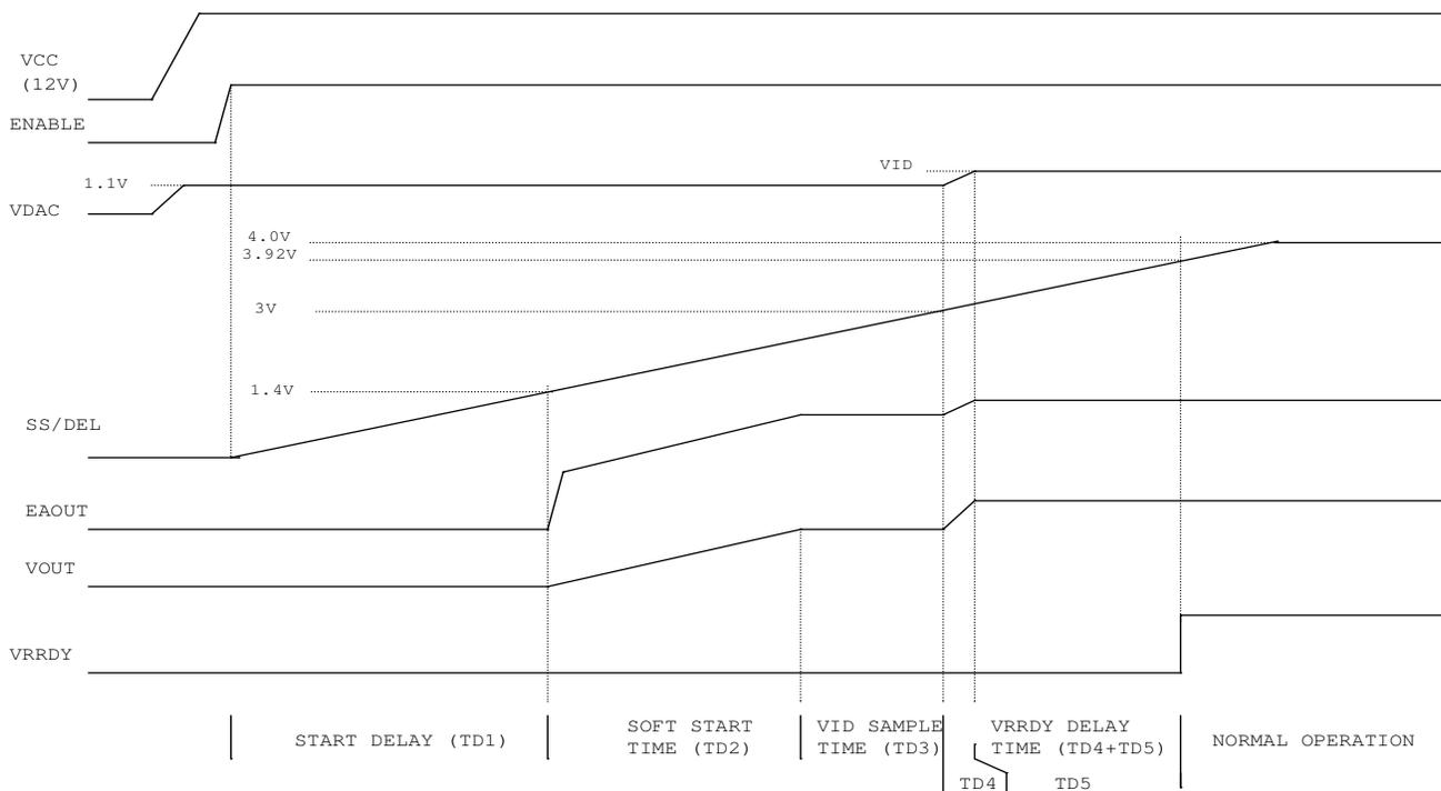
Figure 9 Start-up sequence of converter with boot voltage
