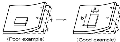
(2) Components location on PCB separation
