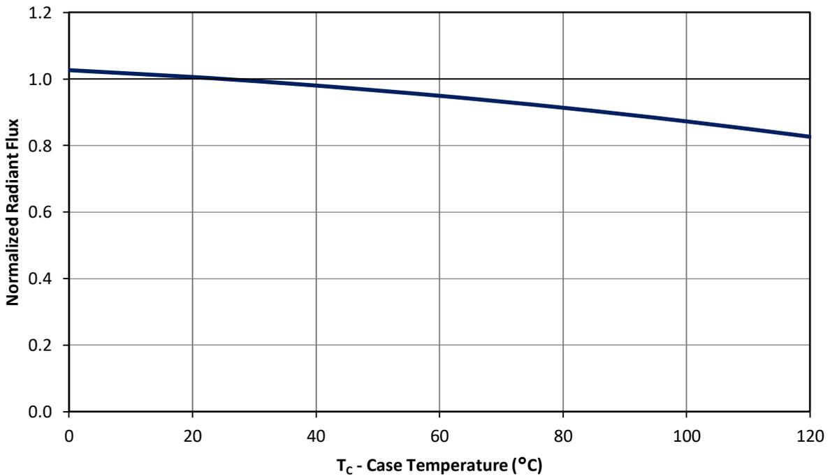
Figure 8: Typical normalized radiant flux vs. case temperature.
