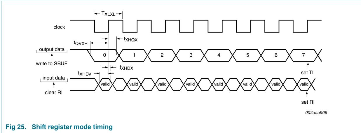
**Fig 25. Shift register mode timing**
