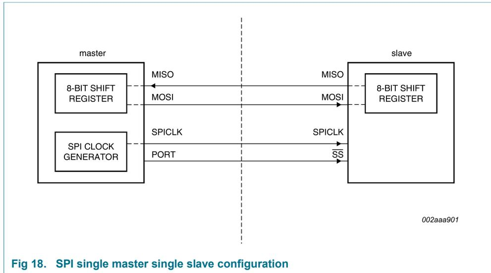
Fig 18. SPI single master single slave configuration
