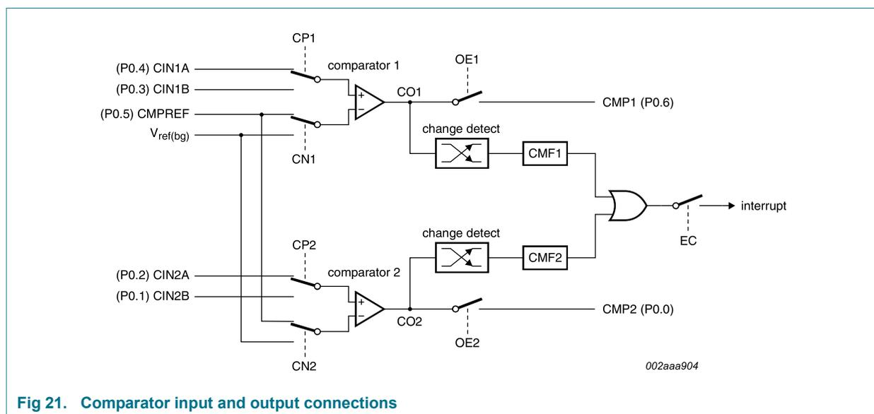
Fig 21. Comparator input and output connections
