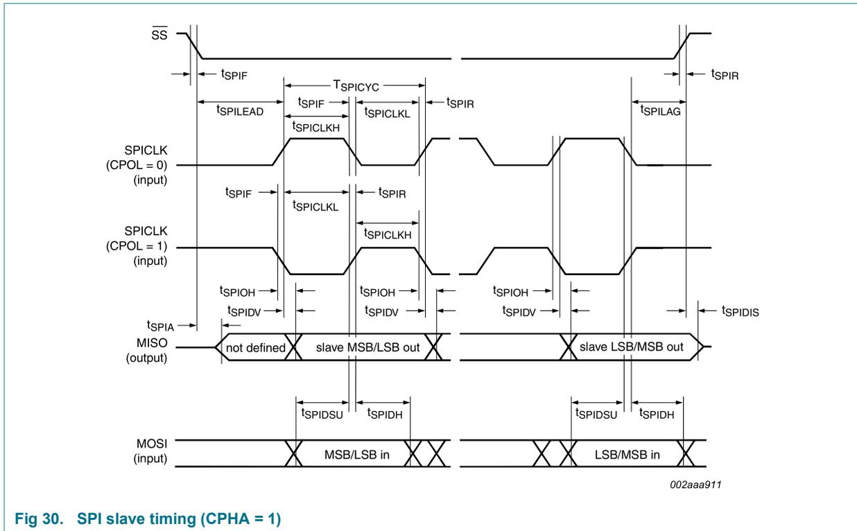
Fig 30. SPI slave timing (CPHA = 1)
