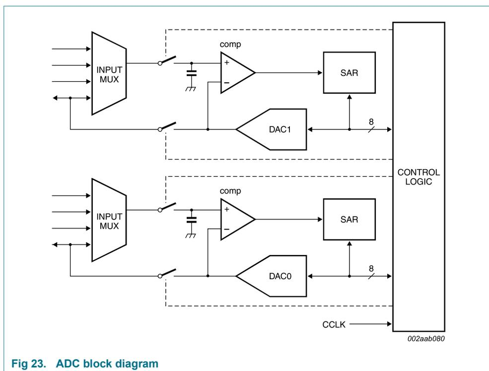
Fig 23. ADC block diagram
