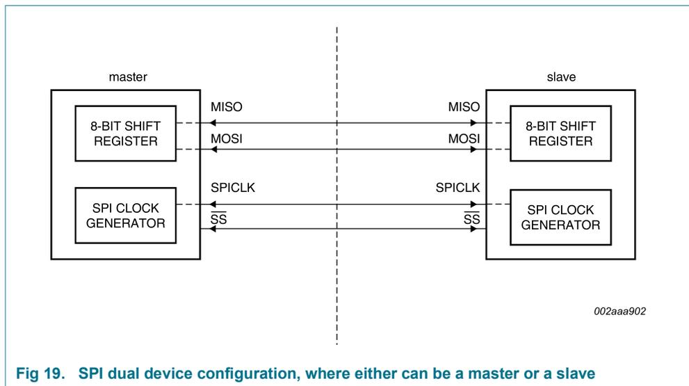
Fig 19. SPI dual device configuration, where either can be a master or a slave
