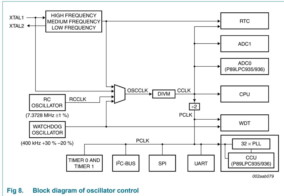
**Fig 8. Block diagram of oscillator control**
