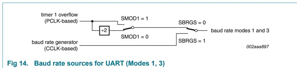
Fig 14. Baud rate sources for UART (Modes 1, 3)
