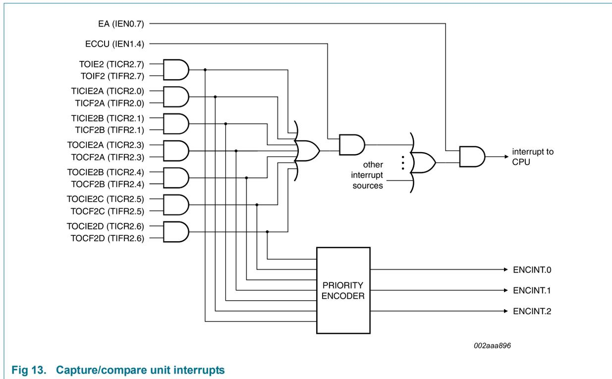
Fig 13. Capture/compare unit interrupts
