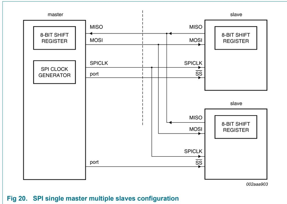
**Fig 20. SPI single master multiple slaves configuration**
