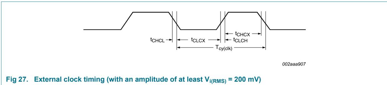
**Fig 27. External clock timing (with an amplitude of at least  $V_{i(RMS)} = 200$  mV)**
