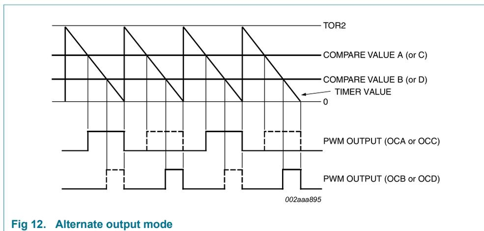
Fig 12. Alternate output mode
