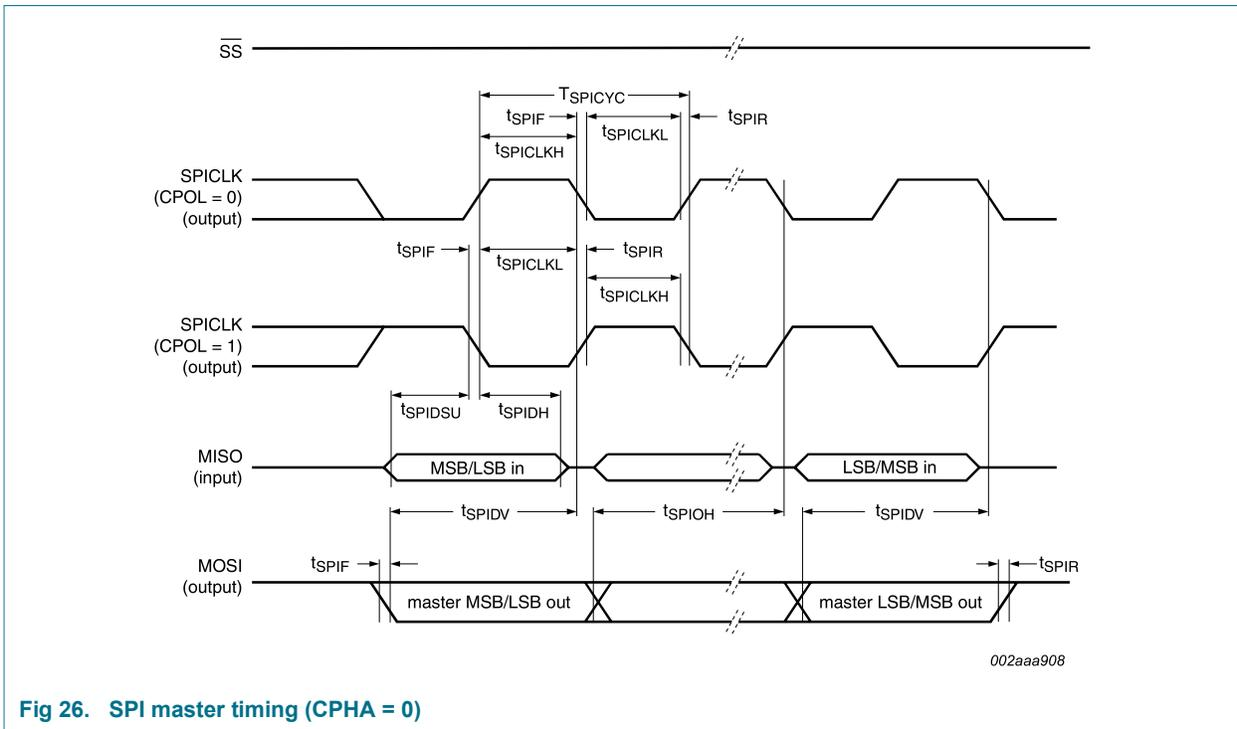
**Fig 26. SPI master timing (CPHA = 0)**
