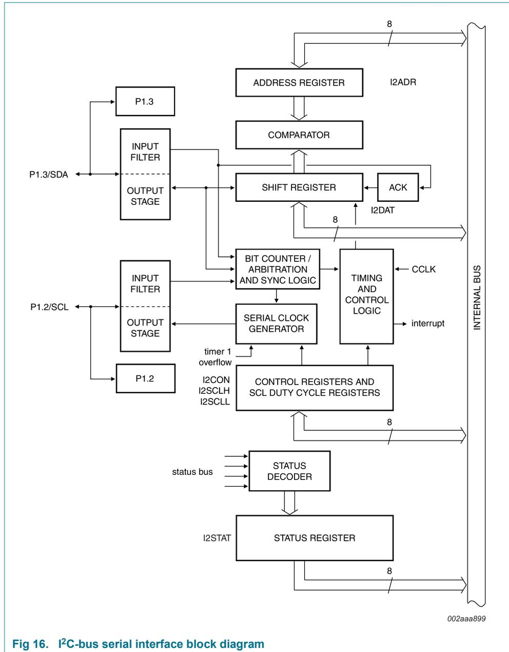
**Fig 16. I<sup>2</sup>C-bus serial interface block diagram**
