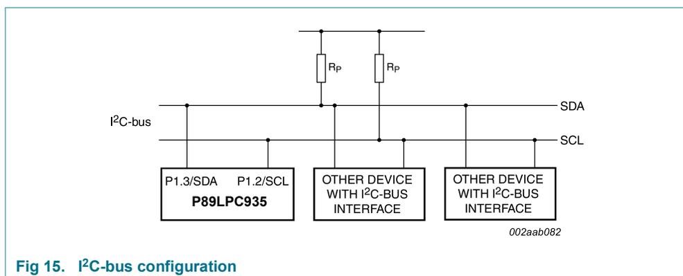
**Fig 15.** I<sup>2</sup>C-bus configuration
