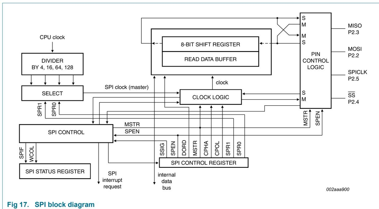
Fig 17. SPI block diagram
