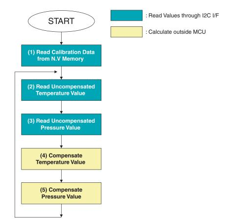
Read calibration data which are contained in internal NVM through I2C.
