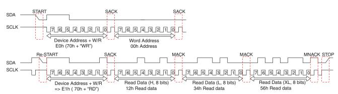
Pressure/Temperature data consists of 24 bits and output as three blocks of 8 bits. Data will be output as H, L and XL order and each 8 bits also output as MSB first.
