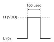
Examples of the reset pulse (reset at the potential of High) Pulse width: 100 µsec. or more
