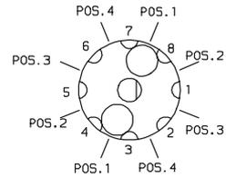
NOTE: Break-before-make contacts. Terminal numbers are molded on bottom of housing. Actuators and contacts are shown in position 1. No common terminal is present. Switching function is provided by movable contacts shorting adjacent pairs of stationary contacts.
